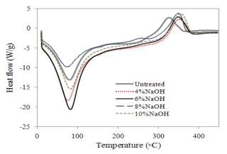
Figure 2. DSC analysis of alkali treated fibre
