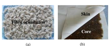
Figure 1. (a) Fibre orientation in the mold; (b) skin attach on the core.
