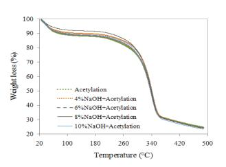
Figure 5. TGA analysis of acetylation treated fibre
