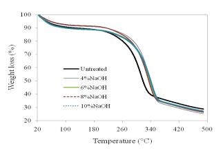
Figure 4. TGA analysis of alkali treated fibre
