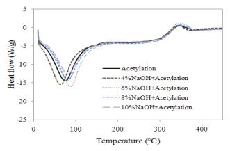
Figure 3. DSC analysis of acetylation treated fibre
