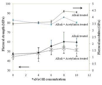
Figure 6. Flexural properties of the composites
