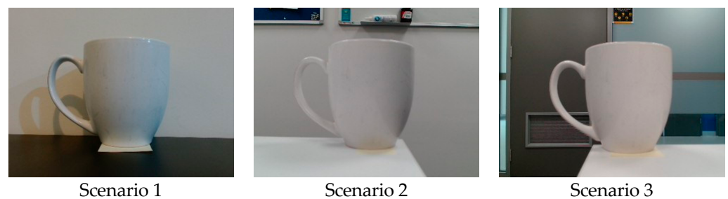
Figure 6. Images of Vessel 1 in different scenarios (camera: Logitech C920e, distance: 20 cm, image resolution: 320 \times 240 ).
