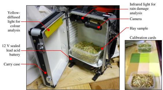
Figure 5. Fodder imaging carry case for quality assessment. *Inset*: Calibration cards used to set image analysis thresholds for colour grading with tubs of grade 60 hay (*top*) and grade 33 hay (*bottom*).
