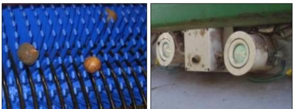
Figure 2. Vision-based macadamia yield monitoring: nuts lodged in pinwheel (*left*) and camera between two lights on the harvester (*right*).
