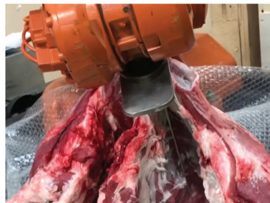
Figure 8. Lamb forequarter ribcage separation (robotic force guided bone following).
