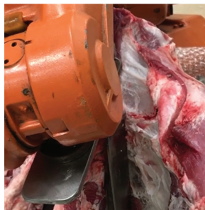
Figure 8. Lamb forequarter ribcage separation (robotic force guided bone following).
