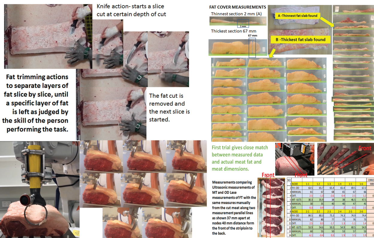
Figure 9. Robotic trimming leaving a uniform layer of specified thickness behind.
