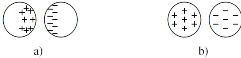
Figure 1.3: (from (Hassan & Stepanyants, 2015)). Electric charge redistribution within two conducting unlikely charged spheres (a) and two unlikely charged spheres with uniformly distributed charges (b).
