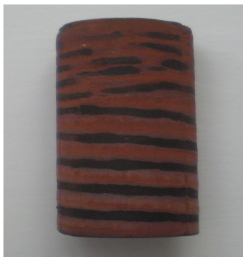
Figure 1.2: A post-combustion trace left by the spinning solid flame on a hollow cylinder.
