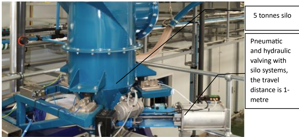
Figure 6.7 Pneumatic and Hydraulic Valving with Silo Systems (Alibaba, 2021)
