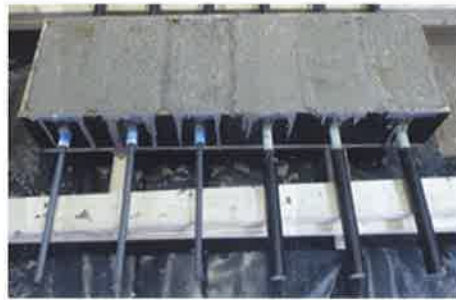
Horizontally cast bond-slip specimens.
