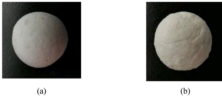
Fig. 3. (a) Spherical mixture of \text{NaHCO}_3 , \text{Ca(OH)}_2 and \text{C}_6\text{H}_8\text{O}_7 and (b) photocatalytic self-healing capsules.
