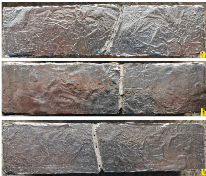
Fig. 9. Samples prepared for the water permeability tests.
