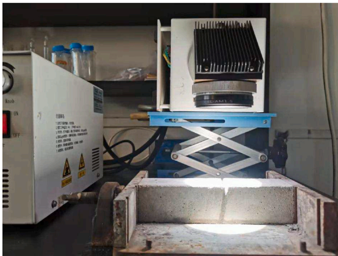
Fig. 6. Irradiation directed to the concrete cracks.
