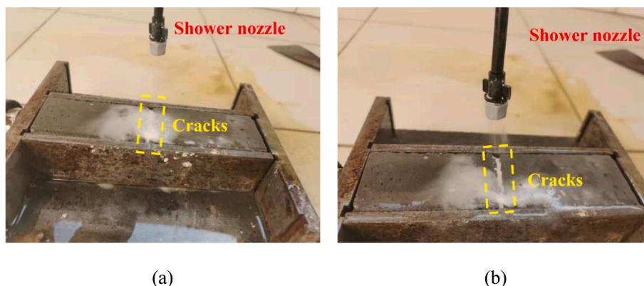
Fig. 7. Cracks (a) at the beginning of spraying and (b) after 3 min of spraying.
