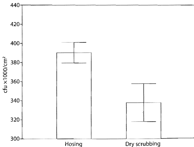
Figure 18.10. Post cleaning bacterial load (mean \pm standard error) of hygiene pavers (colony forming units per cm 2 ): hosing vs. dry scrubbing ( P=0.12 ), 3 hygiene pavers per treatment.
