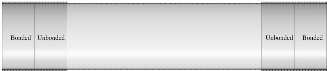
Fig. 15. A schematic of bonded and unbonded partition considered in the PIP system.
