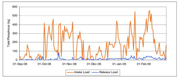
Figure 4: Luggage Point AWTP - daily intake and release loads of total phosphorus (kg).
