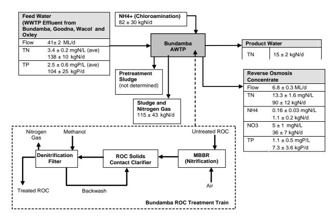
Figure 3: Nutrient mass balance for Bundamba AWTP – August 2008 to February 2009.
