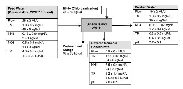
Figure 2: Nutrient mass balance for Gibson Island AWTP – August 2008 to February 2009
