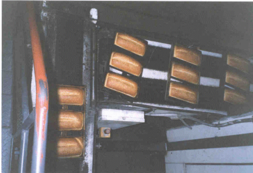
Figure B.13: Tins exiting oven and moving onto conveyor
