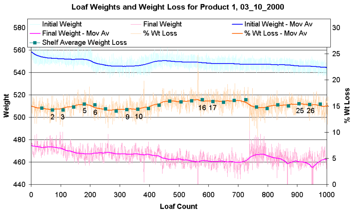
Figure 5.13: Weight loss for the first one thousand loaves of Product 1, 03/10/2000. The numbers on the Wt Loss series refer to the shelf number.
