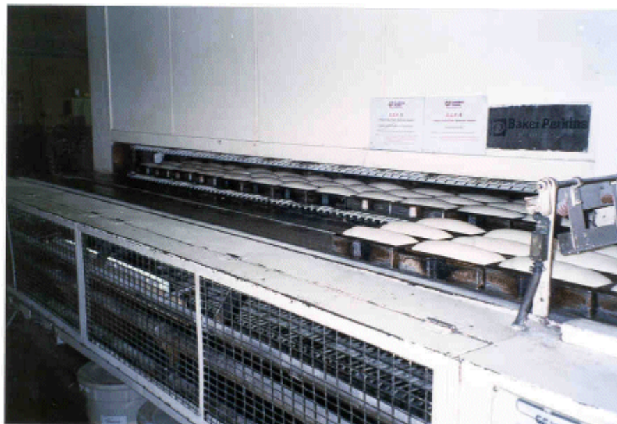
Figure B.10: Tins exiting proofer
