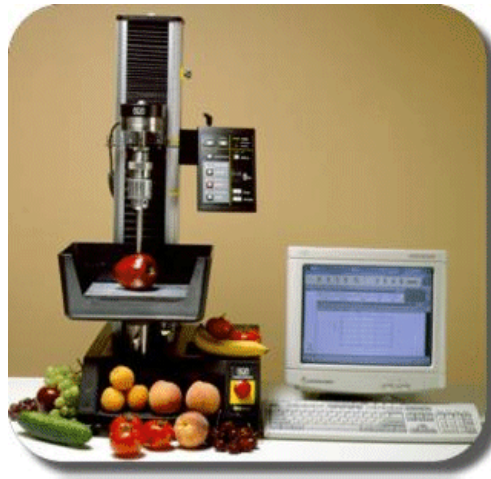
Figure 2.3: An example of an Instron Universal Testing Machine (from the Instron website, http://www.Instron.com )
