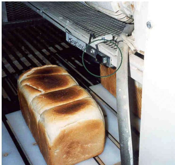
Figure 3.14: Photo of one of the overhead loaf sensors at the conveyor split
