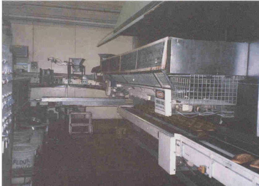
Figure B.11: Oven entry and exit section
