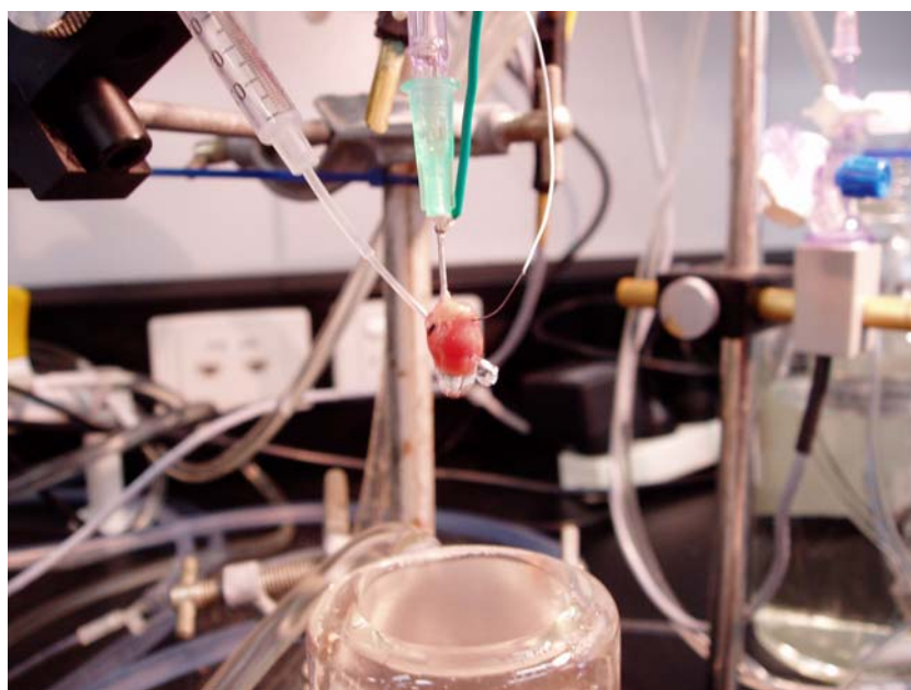
Figure A2.2: Final Langendorff set up, with heating coil to ensure correct perfusion fluid temperature.
