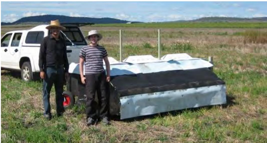
Figure 2.3: Three metre spot sprayer developed for plant identification and spot spraying at the NCEA (McCarthy et al. 2012). Camera and lights are mounted under white plastic covers with a light-restricting cover around the sprayer.
