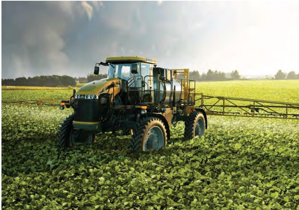
Figure 1.3: Agchem high clearance sprayer (Croplands Australia Ltd 2013).
