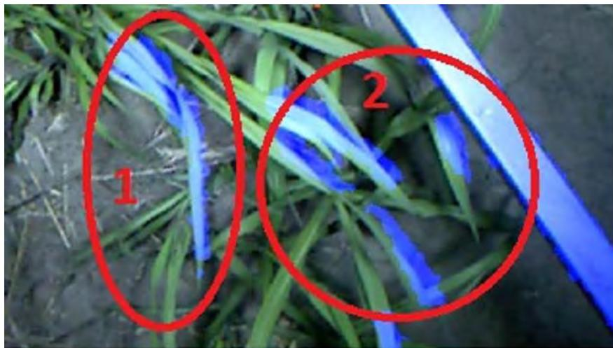
Figure 4.7: Depth image superimposed onto the blue channel in the colour image of sugarcane. The superimposed red circle labeled 1 shows correctly positioned (overlaid) leaves in the depth and colour image. The superimposed red ellipse labeled 2 highlights incorrectly positioned (overlaid) leaves in the images.
