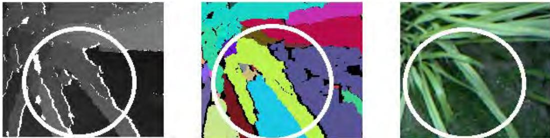
Figure 5.10: Image showing the depth image, segmented image and colour image associated with each other. The white ellipse highlights two separate leaf components that overlapped in colour and height and therefore are the one component.
