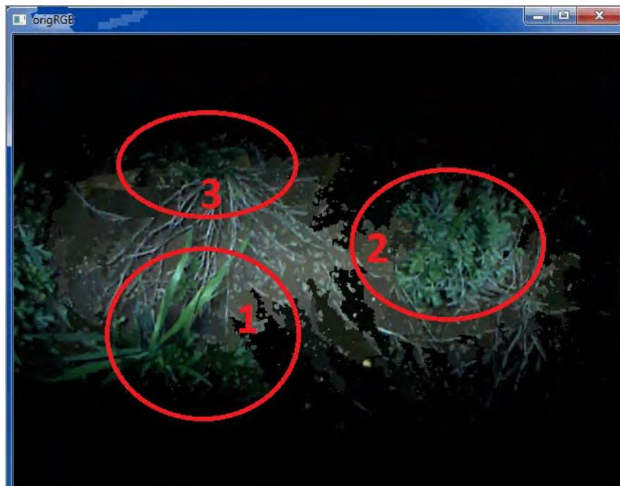
(b) Split and merge segmentation technique applied to a colour image 5.1(a).
