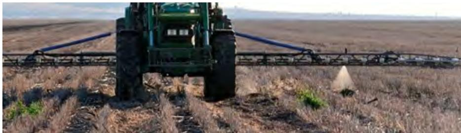
Figure 1.8: Boomspray equipped with Weedseeker technology (reproduced from Cropoptics Australia (2012)).
