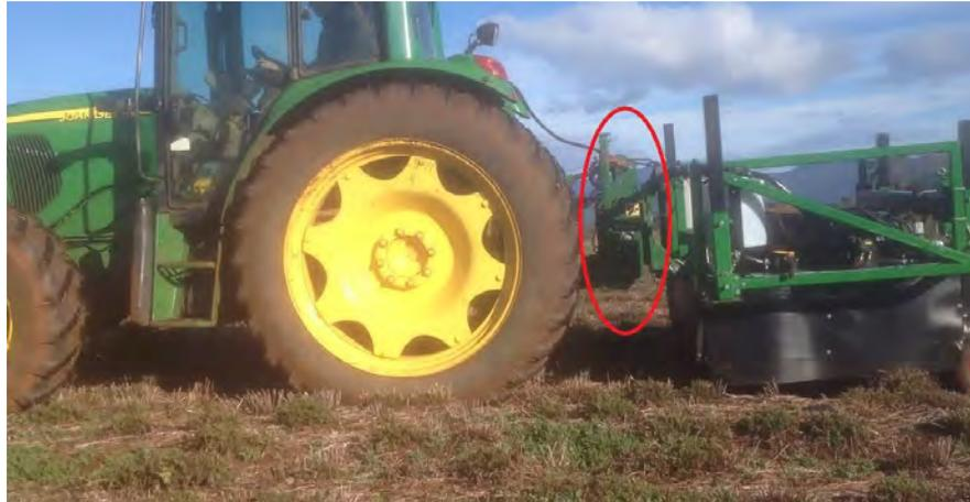
Figure G.1: Image of side shift hitch (in the red ellipse) in position between the tractor at the front and the implement at the rear.
