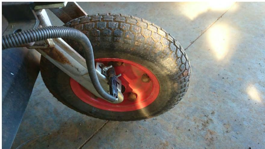
Figure 3.1: The magnetic wheel speed sensor is shown with the sensor and the magnets mounted on the wheel. Each time the magnet passes the sensor, a pulse is created.
