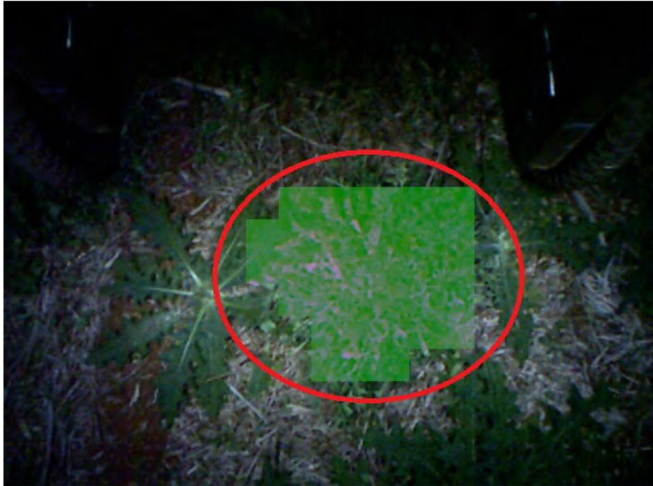
Figure 6.10: Image with 34 LBP sliding windows of identification (highlighted green squares on the pyrethrum plant in the red ellipse).
