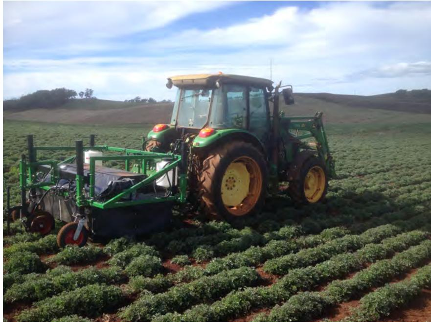
Figure C.2: Tractor and experimental NCEA prototype spot spray system in a crop of first year growing pyrethrum April 2014.
