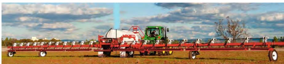
Figure 1.9: Boomspray equipped with Weed-It technology (reproduced from Croplands Australia Ltd (2013)).
