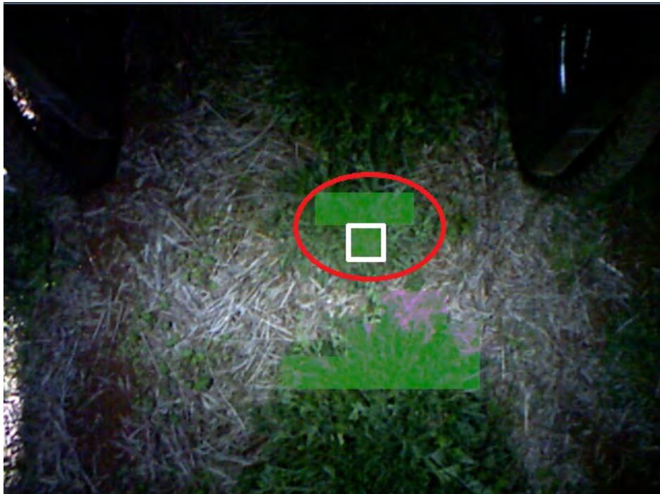
Figure 6.9: Image with four LBP sliding windows of identification (highlighted green squares on the pyrethrum plant in the red ellipse). The green block bordered by white inside the red ellipse demonstrates the size of a  $32 \times 32$  pixel window.
