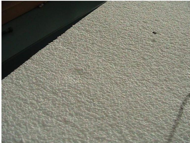
Figure 3. 5 Surface of a raw high density expanded polystyrene
