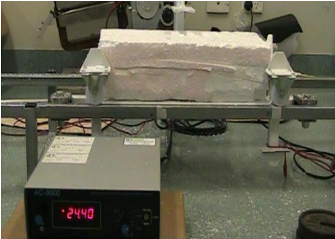
Figure 3. 8 Test set-up for cutting force resistance on powered disk blades
