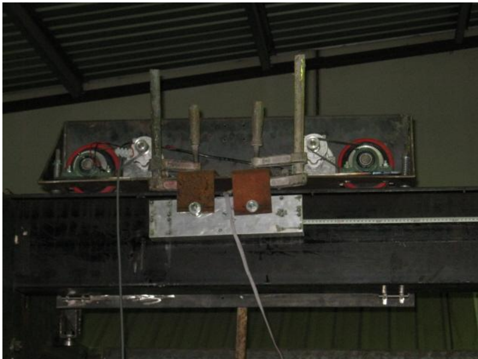
Figure 4. 23 The fabricated lateral slider with direct drive traction unit and the designed transducer that read patterns from a two millimetres surveyor tape
