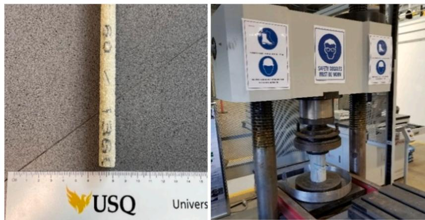
(a) Sand-coated GFRP bar (b) Compression test.
