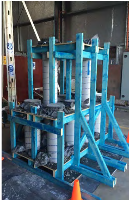
Fig. 5. Wooden framework and plastic formworks with cast column specimens.
