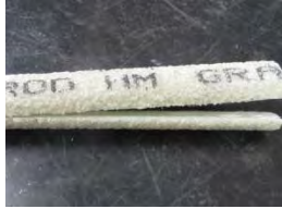
Figure 6. Interlaminar shear failure of GFRP bars (21 °C to 80 °C)
