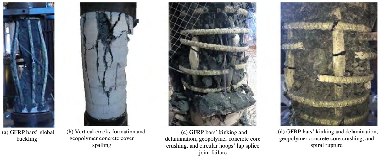
Fig. 9. Different failure mode configurations of the column specimens.
