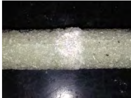
Figure 5. Crushing of the resin and fibre of GFRP bars (21 °C to 80 °C)
