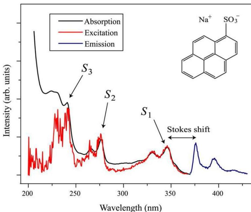
**Figure 1.17** Absorption, excitation and emission spectrum of pyrene sulfonic acid (pictured top right). Three excitation states are observed for the molecule. Fluorescence occurs when the molecule shifts from the lowest excitation state ( $S_1$ ) to the ground state, resulting in a Stokes shift (reproduced from Learmonth, Kable & Ghiggino 2009).
