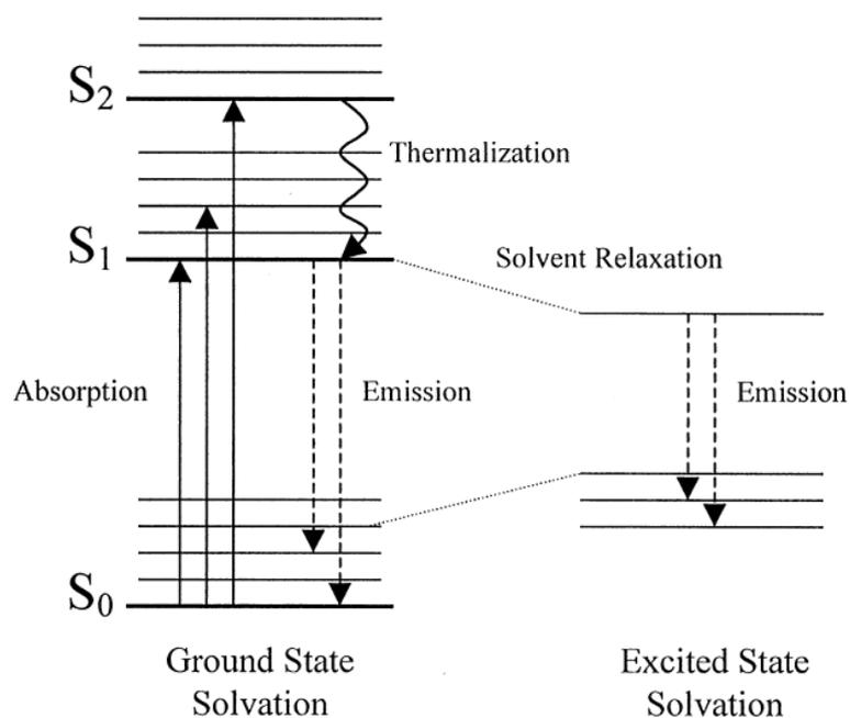
**Figure 1.16** Simplified Perrin-Jablonski energy level diagram showing absorption (—) and emission (---) processes as well as thermalization and solvent relaxation (reproduced from Croney, Jameson & Learmonth 2001).
