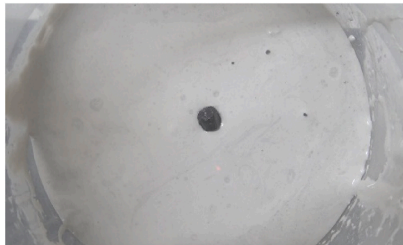
Fig. 6. Partial immersion of encapsulated dyed sodium silicate accelerator to experimentally validate the underlying mechanisms involved in the studied set-on-demand approach for buildability enhancement in concrete 3D printing.
