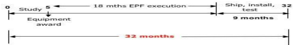
Figure 5.6 Modular LNG Schedule; (Chart Energy & Chemicals Group, 2013)
