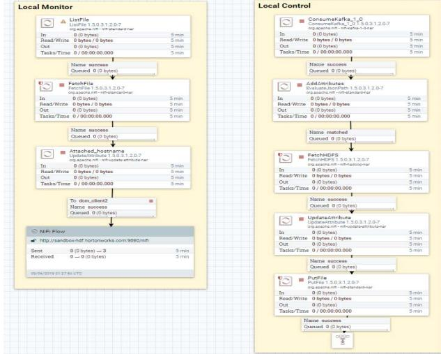
Fig. 4. NiFi Data flow of Monitor and Executor of DCM Edge
