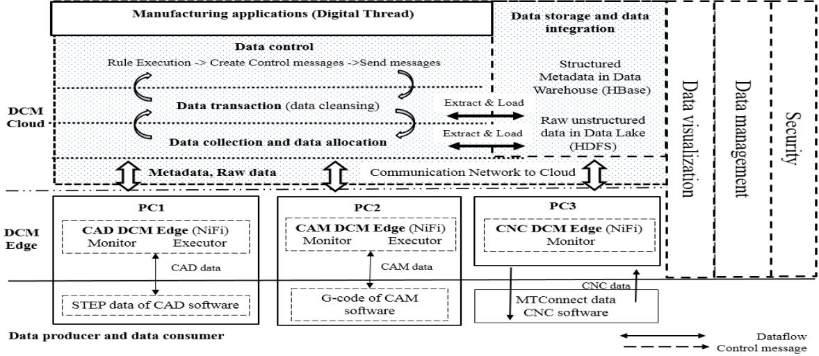
Fig. 2. Digital thread application with DCM methodology
