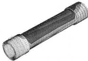
Figure 12. FEA model of the cylindrical specimen
