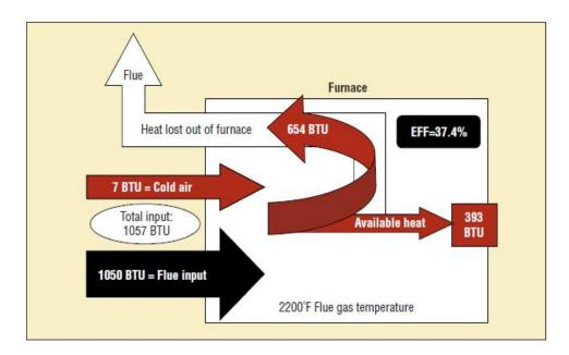
Figure 4. Efficiency of the heating system without EGR (Kraus and Barraclough, 2012).
