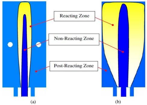
Figure 3. Closed furnace reacting zone for (a) conventional and (b) MILD combustion (Li and Mi, 2011)
