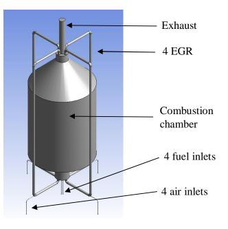
Figure 6. Open furnace with 4 EGR and top chamber opening.
