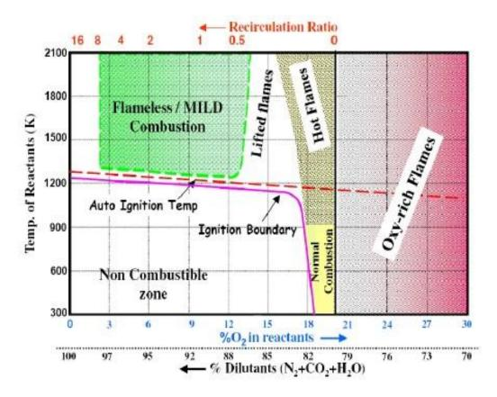
Figure 1. Schematic regime diagram for methane-air JHC flames (Rao, 2010).
