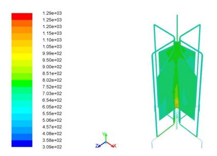
Figure 7. Combustion temperatures for low calorific value gas.
