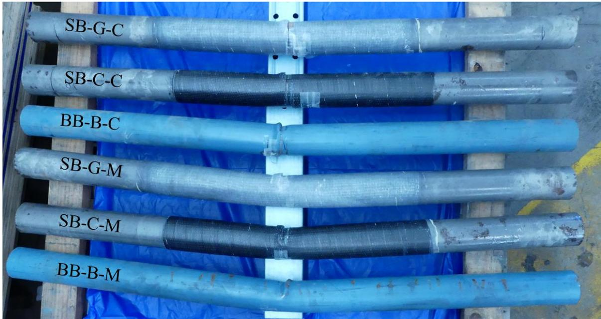
Figure 6: Tested bare, CFRP and GFRP strengthened CHS members.
