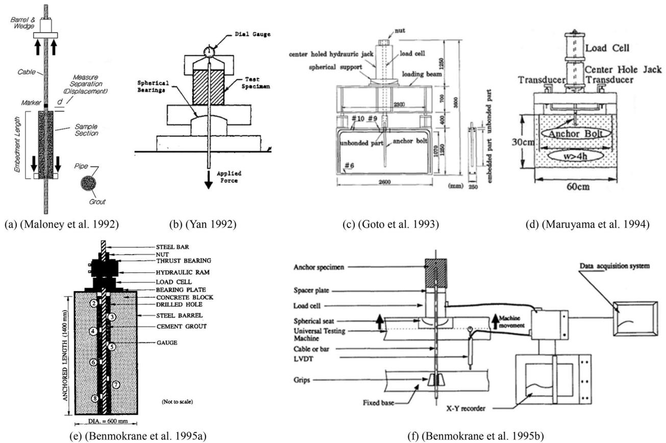
Fig. 8 Structures of the developed SEPT rigs in the 1990s
