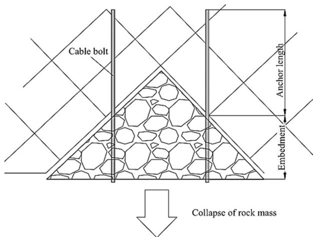
**Fig. 12** A normal failure form of the tendon in the field condition (Chen et al. 2018)
