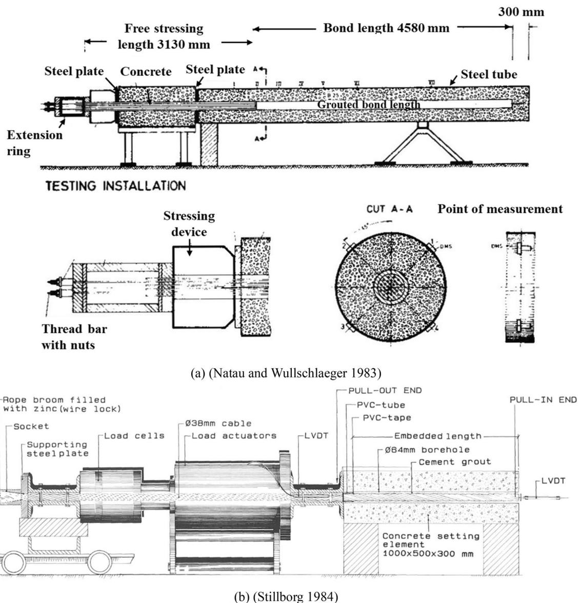
Fig. 7 The structures of the developed SEPT rigs in the 1980s
