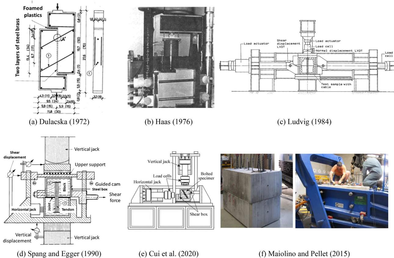
**Fig. 19** Developed apparatuses allowing angle SST
