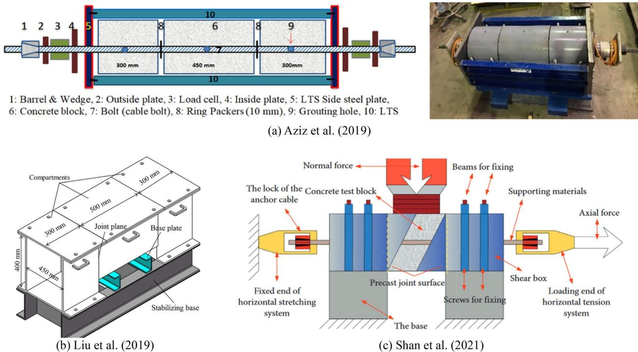
Fig. 18 Perpendicular DST experimental set-ups proposed in the recent years
