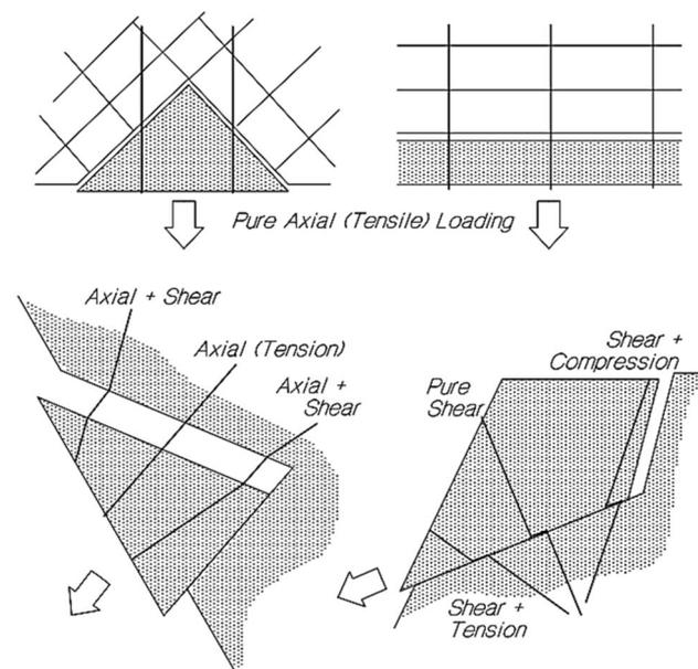
**Fig. 1** A schematic view of different loading modes on tendons in the field condition (Hutchinson and Diederichs 1996)
