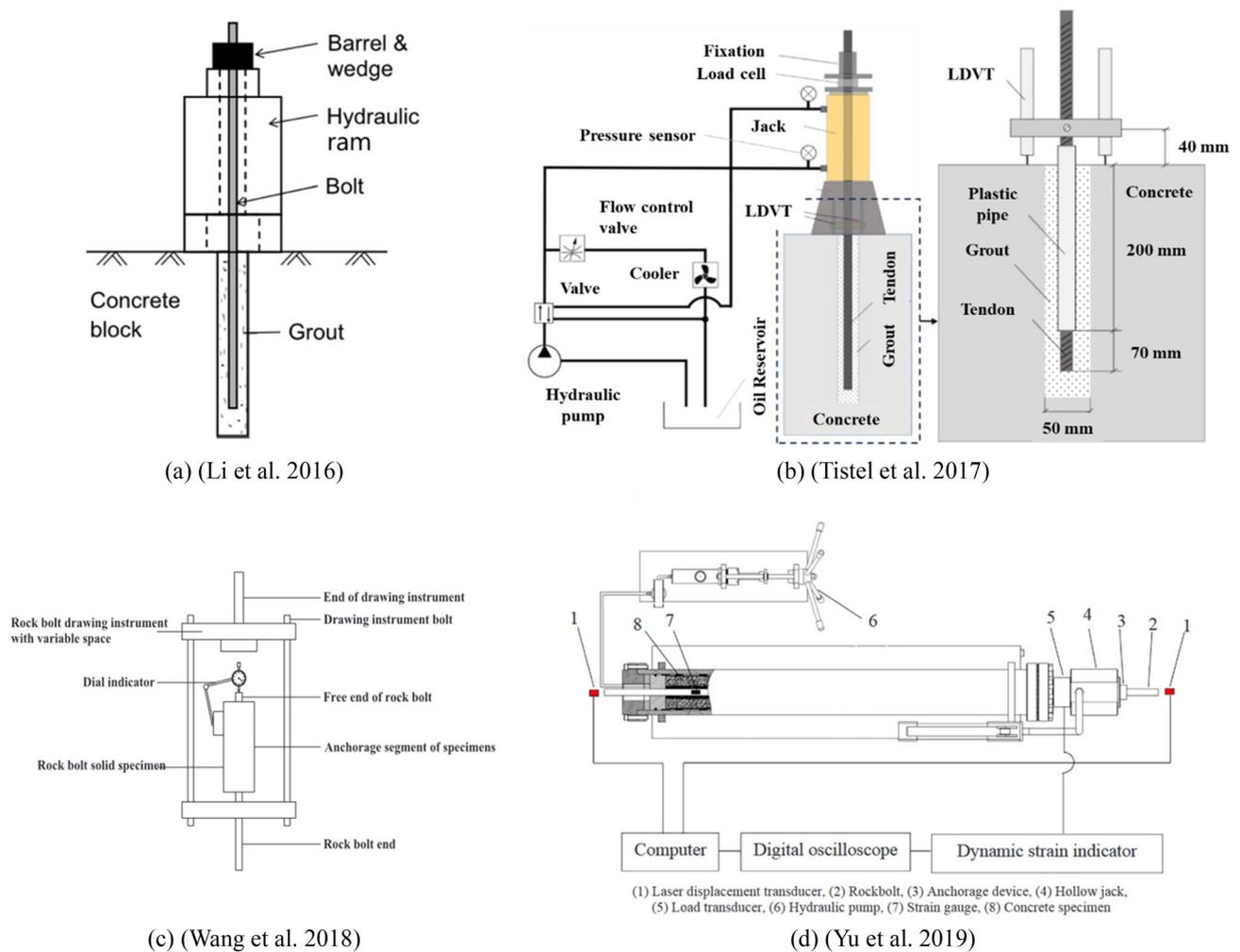
**Fig. 10** The structures of the developed rigs for pull-out testing in the 2010s
