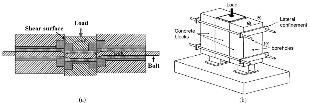
Fig. 16 The DST set-up, adapted from **a** Haile et al. (1995) and **b** Ferrero et al. (1997)
