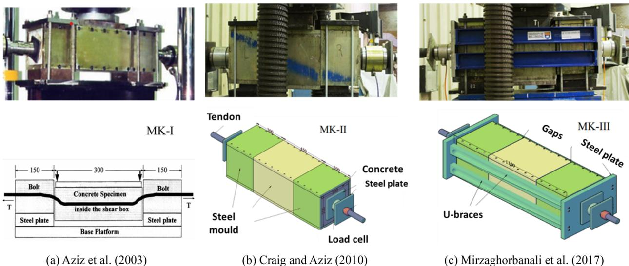
Fig. 17 Perpendicular DST experimental set-ups proposed in recent years
