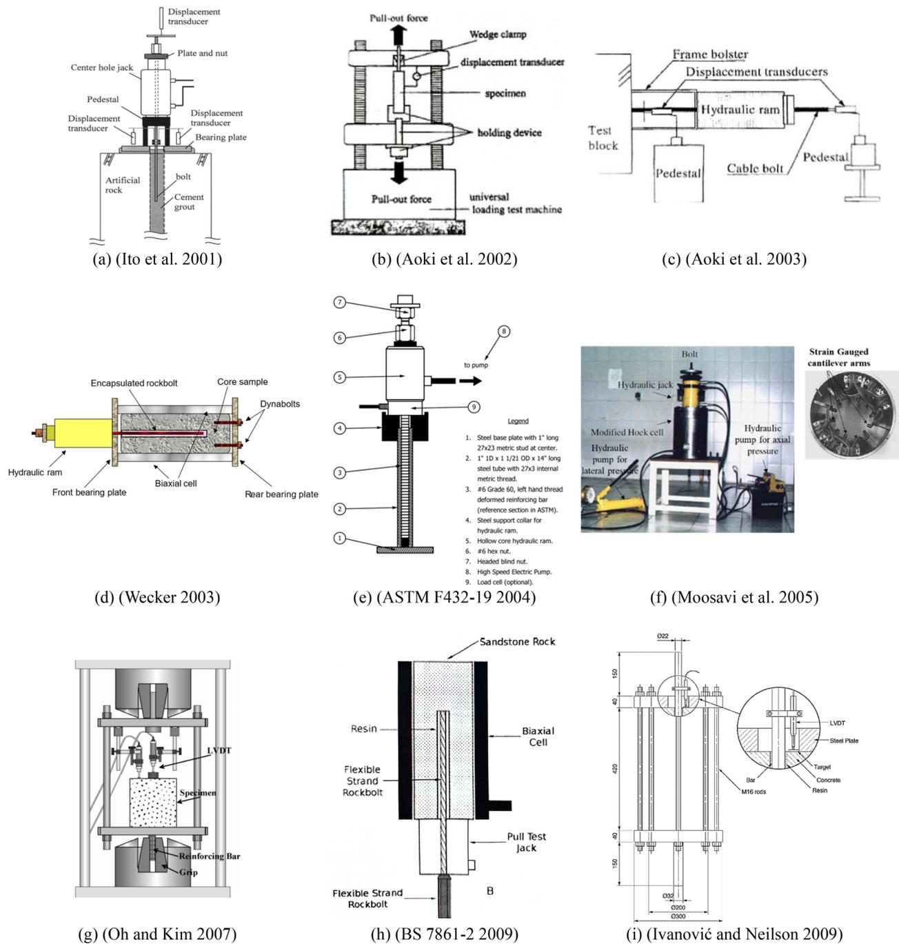
**Fig. 9** The structures of the developed apparatuses for pull-out testing in the 2000s
