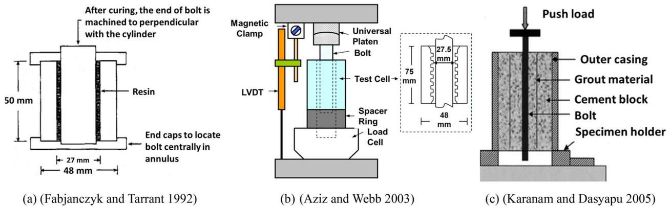
Fig. 3 The structure of apparatuses introduced for push-out testing
