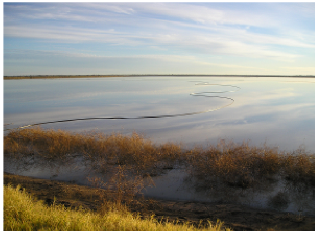
Figure 7: Application of chemical monolayer at the 120 hectare storage at Cubbie Station, Dirranbandi Qld
