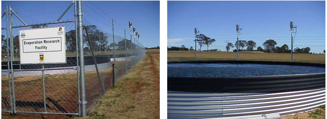
Figure 17: Evaporation Research Facility based at NCEA, USQ. The experimental trial consists of three lined 10 m x 0.8 m deep tanks which are being used to accurately assess the effectiveness of different evaporation control methods.
