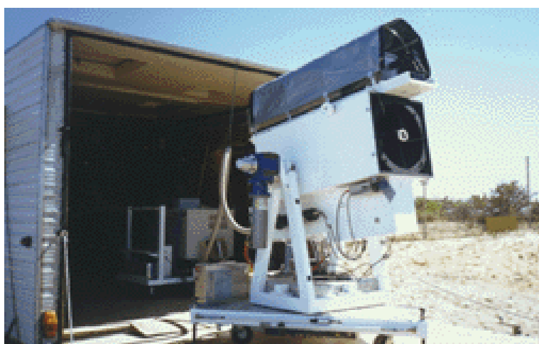
Figure 21: Truck transportable LIDAR machine. The technology uses a scanning UV laser to detect humidity fields and thus deduce total evaporation rates over water bodies
