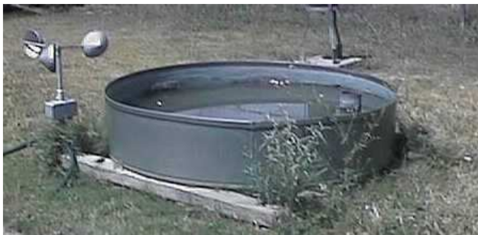
Figure 15: Typical evaporation pan with weeds and no bird guard. The pan is also not filled to the top so there will be significant errors associated with the aerodynamics of the lip
