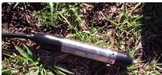
Figure 8: The Druck 4030 Pressure Sensitive Transducer (PST) unit
