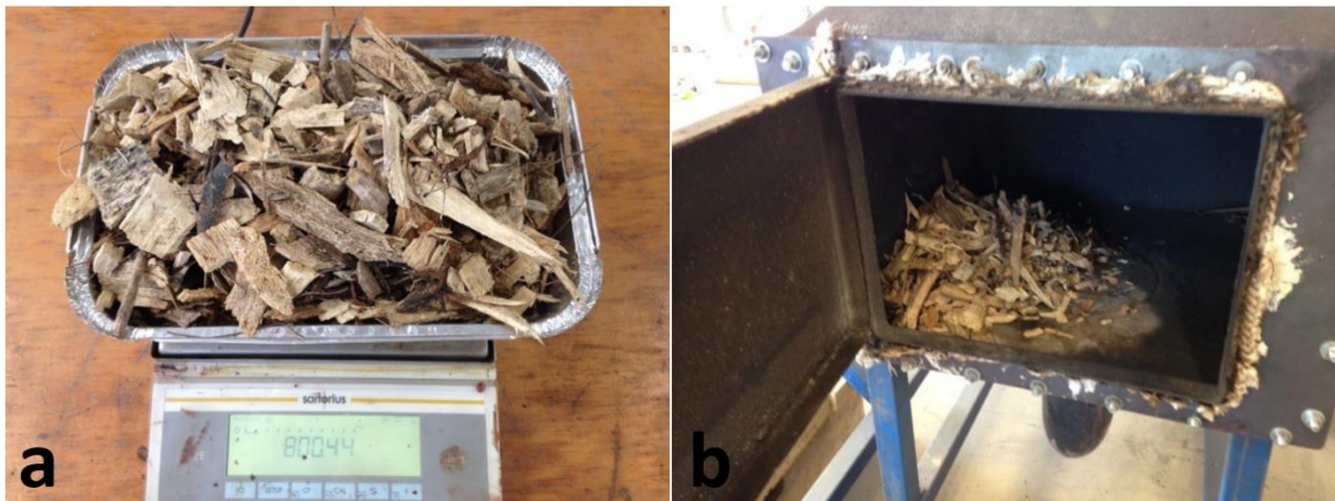
Figure 6 Hardwood mulch applied as feed in generator: a) 800 g hardwood mulch; b) hardwood mulch in the generator.
