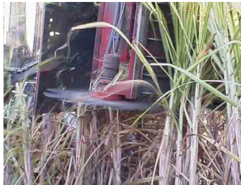
Figure 7.17: Topper removing leafy waste material from upper section of cane stalks
