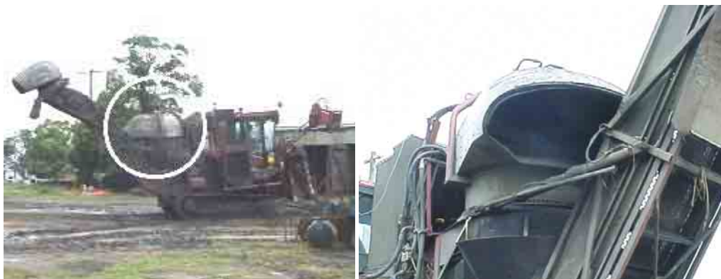
Figure 5.1: Extraction chamber indicated (left) and a closer view of hood chute
