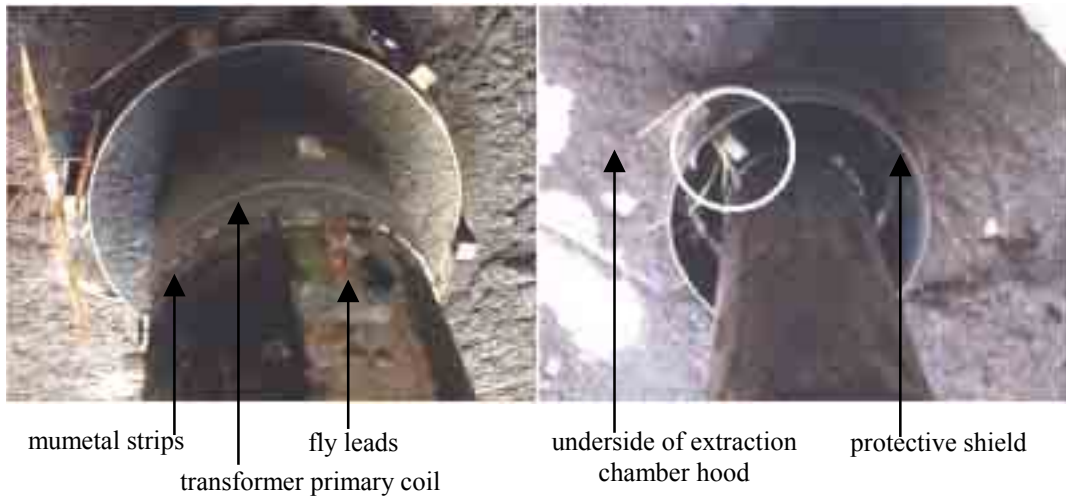
Figure 5.10: First concept field trials of the rotating transformer without (left) and with stationary cylindrical shield. A circle in the right-hand picture has indicated the pick-off device
