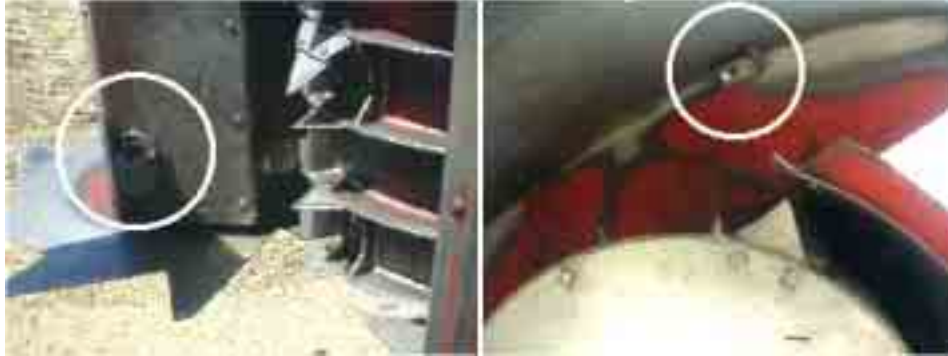
Figure 7.5: Manufactured camera box mounted on topper in two indicated positions: (a) at cutting interface, and (b) back of hood*
