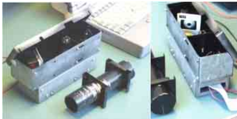
Figure 7.12: Spectrometer test rig with cuvette in position in box, and the collimator is in the foreground
