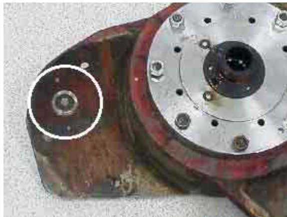
Figure 5.7: Transducer mounted in hub flange
