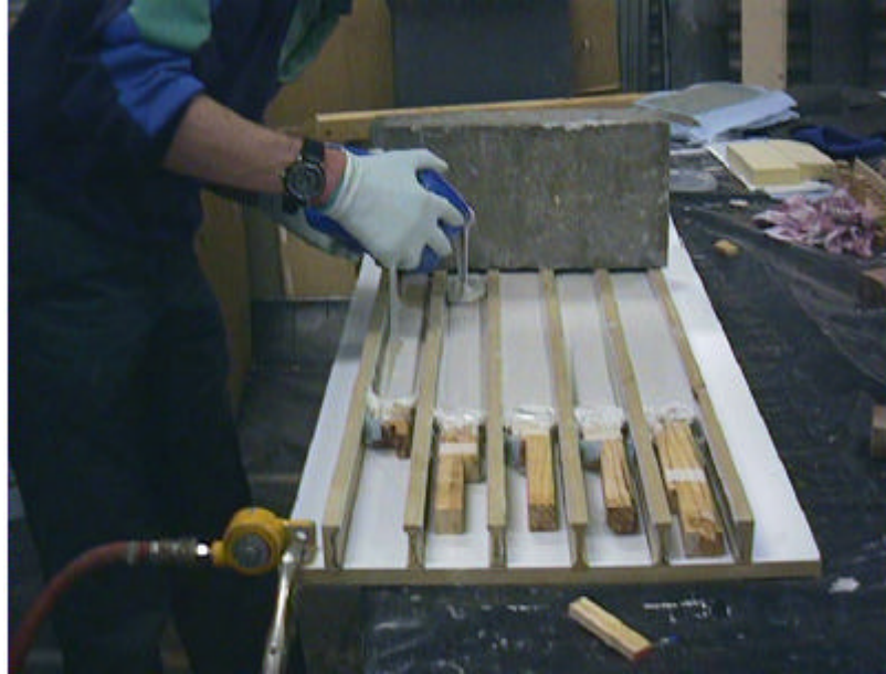
Figure 5.11 Form and pour beam production
