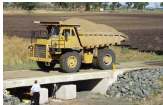
Figure 1.5 Ten metre vehicular bridge undergoing testing in Toowoomba, Queensland
