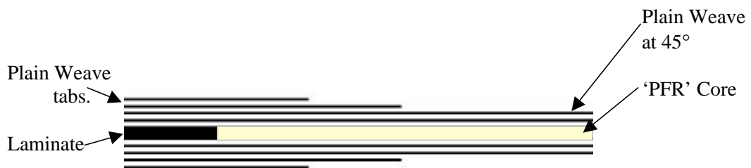
Figure 7.23 Section geometry of web shear specimens
