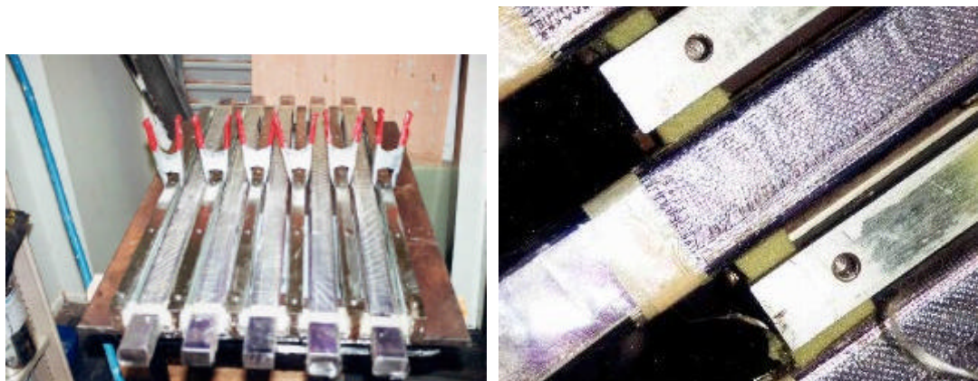
Figure B.3 Mandrels and laminates in mould
