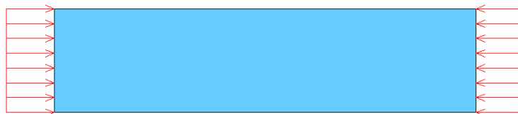
Figure 6.12 Stresses upon the flange
