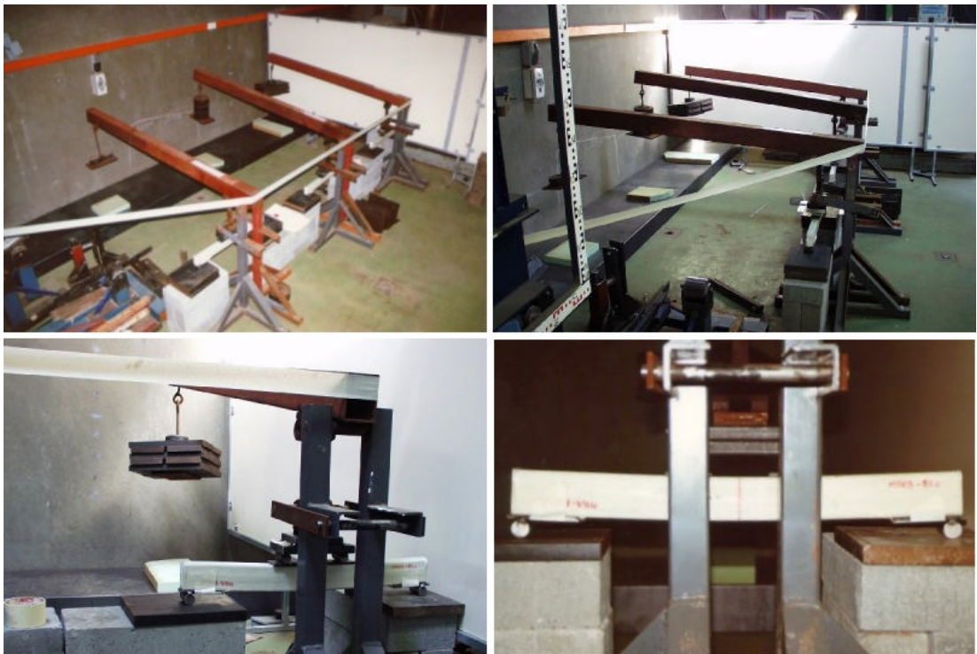
Figure 7.44 Beams undergoing sustained loading
