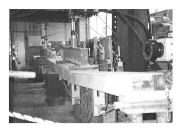
Fig. 3—Testing of continuous beam specimen.
