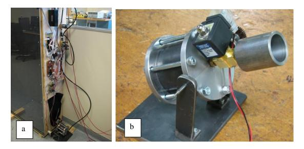
$\label{eq:Figure 3: Annotated photographs of the (a) range and (b) canon used in the model firing range \\ remote experiment$
