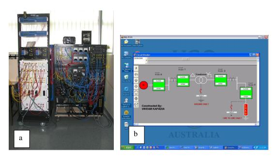
$\label{eq:controlled} \textbf{Figure 2: SCADA controlled network fault simulator. The (a) hardware under (b) software control. }$
