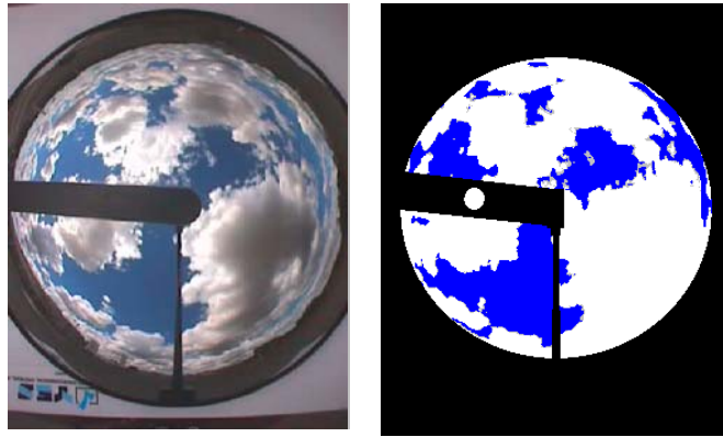
Figure 1: An example unprocessed and processed image from the TSI. The white circle on the shadow band is the position of the sun.
