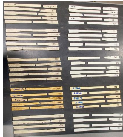
(b) All skin samples tested after 7 months (Hemp skin-left side, PET skin-right side with five different environments)
