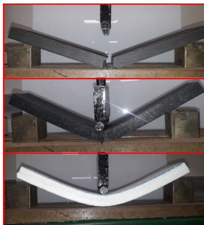
Figure 3.3. Failure pattern of cores (Wood, Plastic, and styrofoam respectively)
