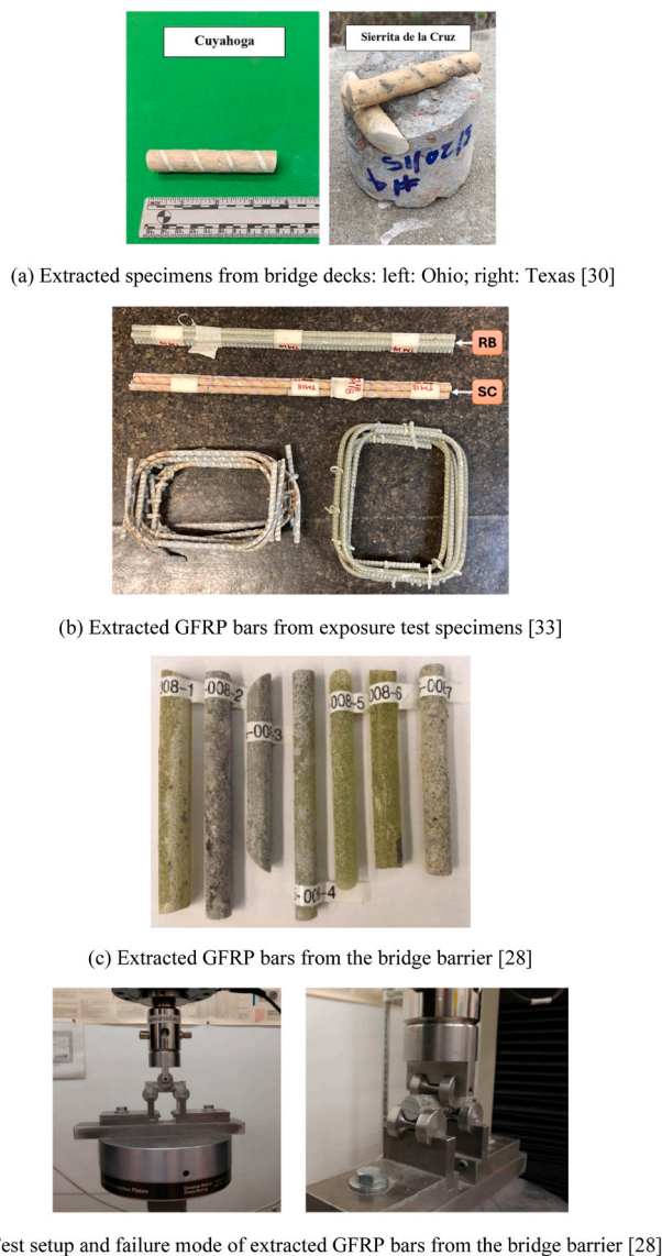
Fig. 11. Extracted specimens from field exposure, test setup, and failure modes.
