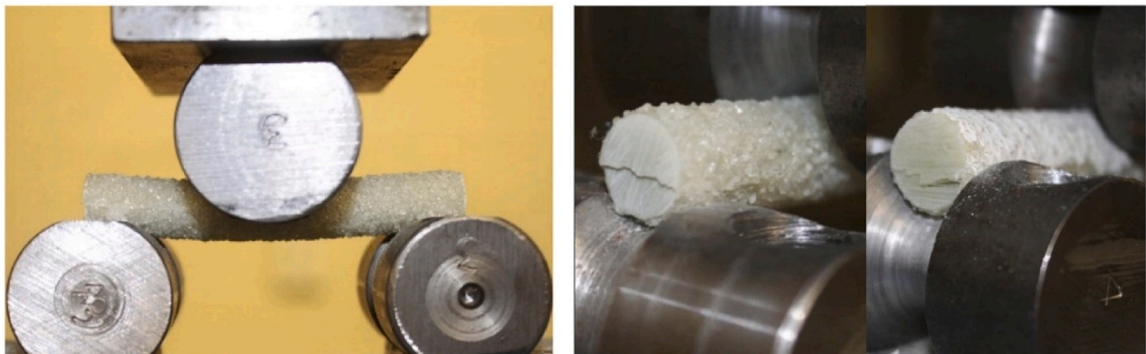
Fig. 10. Test setup and failure mode of laboratory specimens [46].
