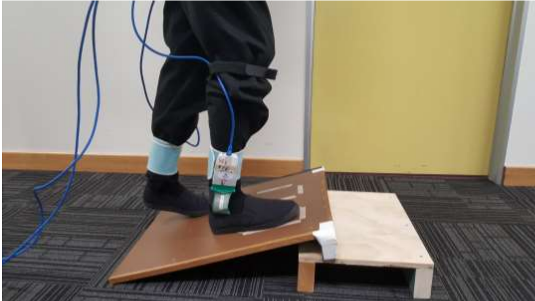
Figure 4.3: An older subject wearing in-shoe 3000E F-scan ® sensors to perform uphill walking task.
