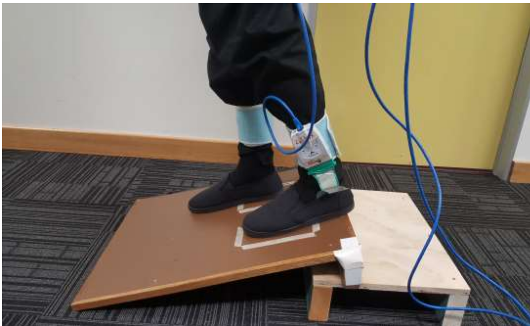
Figure 4.4: An older subject wearing in-shoe 3000E F-scan ® sensors to perform downhill walking task.
