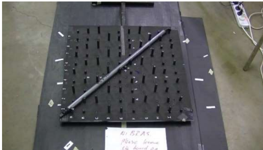
Figure 6.2: Camera calibration target board “test-field”.
