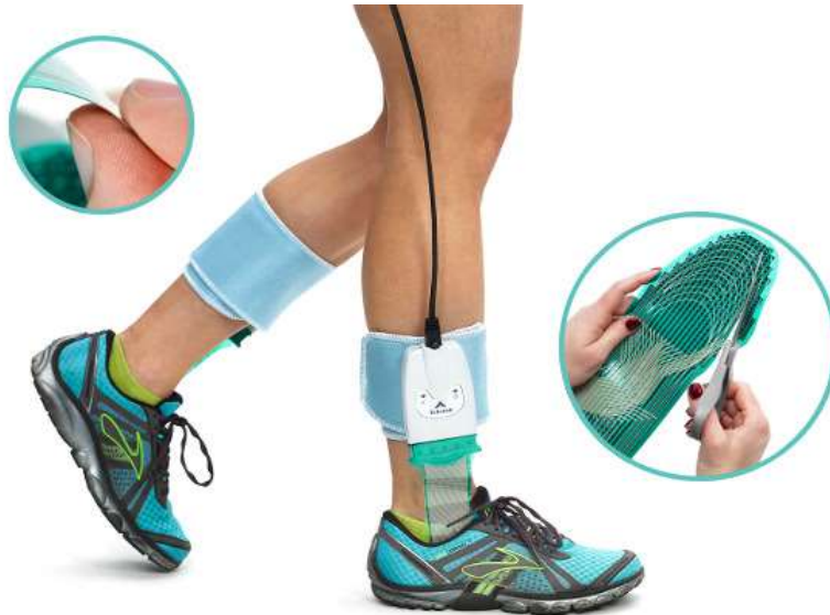
Figure 2.11: F-scan pressure insoles systems attached to human lower limb, picture adopted from the website of Tekscan company (Tekscan, South Boston, MA, USA).
