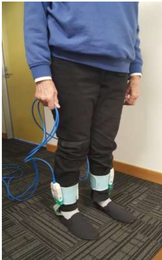
Figure 4.2: An older subject wearing in-shoe 3000E F-scan ® sensors to perform level walking condition.
