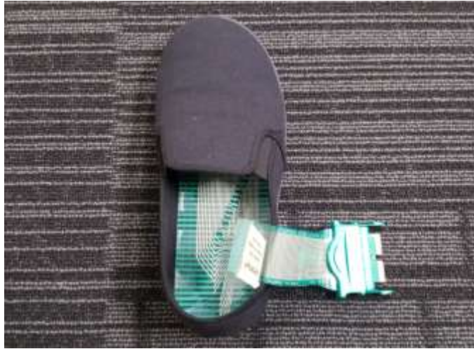
Figure 4.1: An in-shoe 3000E F-scan ® pressure sensor (Tekscan, Boston, MA) system.
