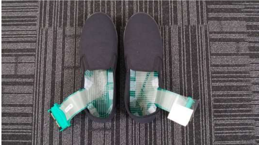
Figure 3.1: An in-shoe 3000E F-scan® sensor of F-scan® pressure (Tekscan, Boston, MA) system.
