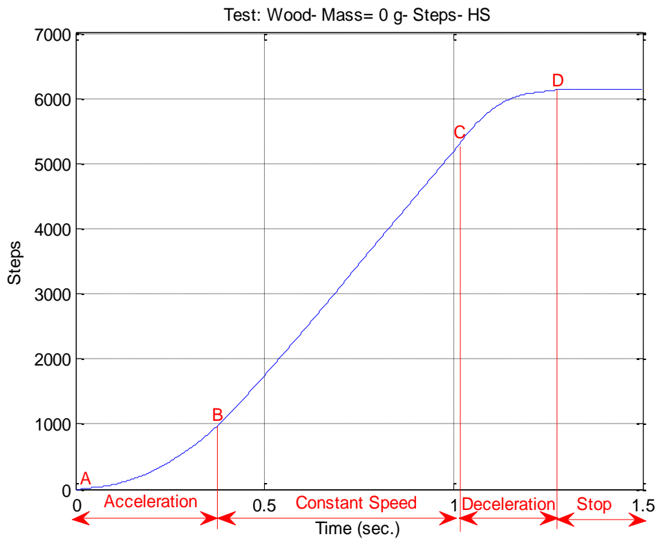
Figure 4.25: Encoder's readings for a speed test (HS = High Speed (12.20 rad./sec. = 116.50 RPM), F_z = 0 N).
