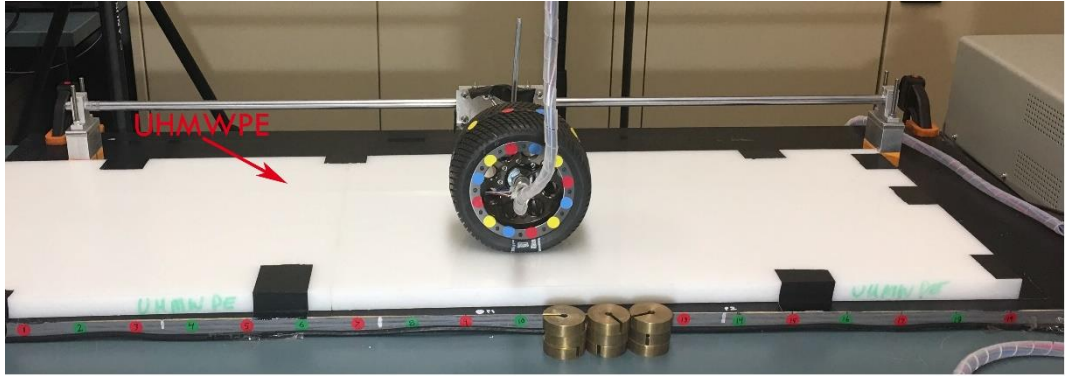
Figure 3.17: Example of the contact surface tests (plastic (UHMWPE)).
