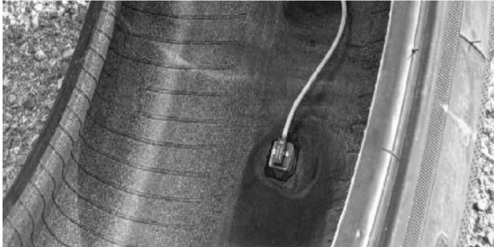
Figure 2.6: In-tyre accelerometer (Savaresi et al. 2008).
