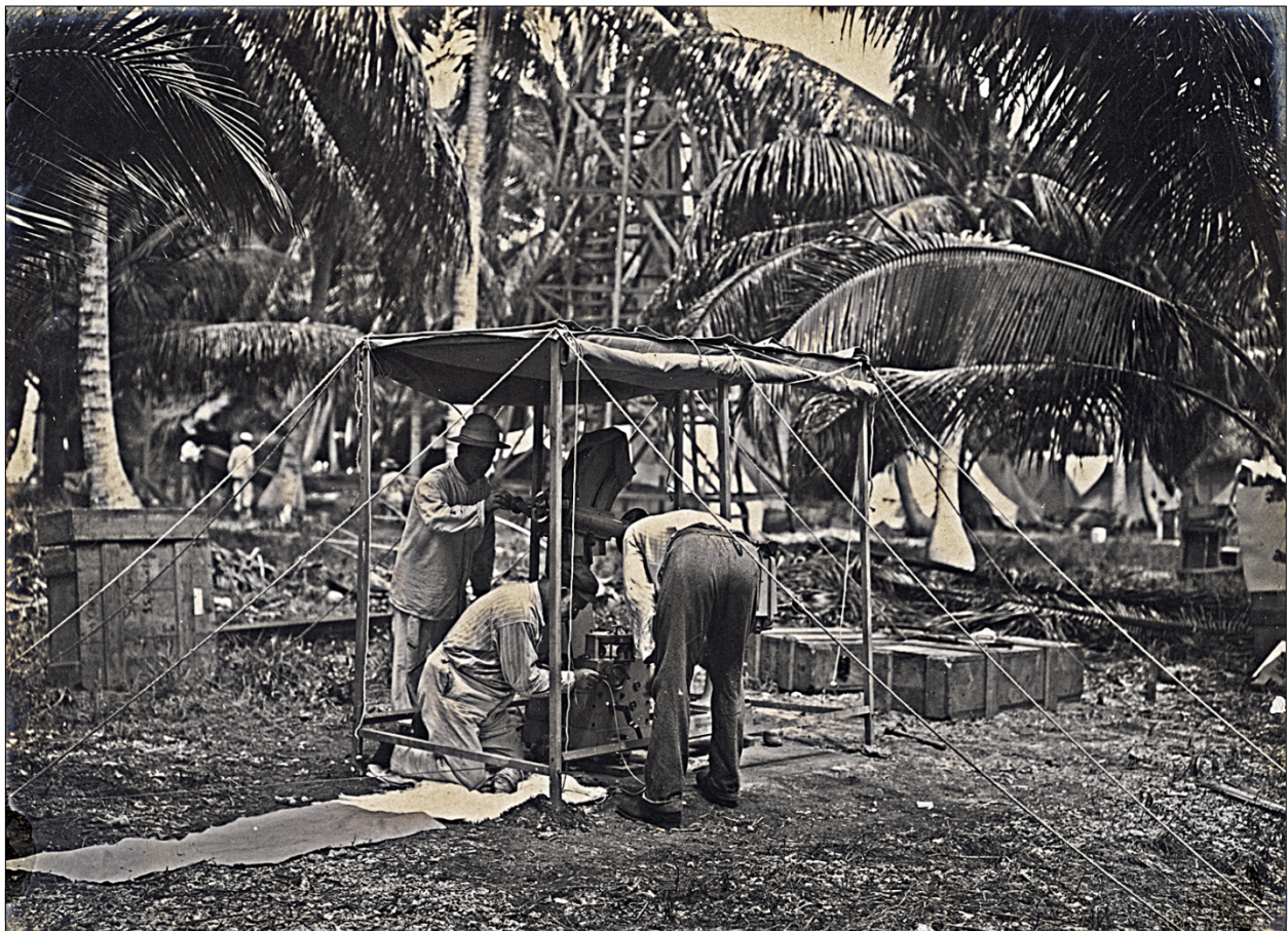
Figure 4: Joseph Brooks adjusting the clock drive for the siderostat with the Lick Observatory tower faintly visible in the background (photo: Henry Winkelmann, courtesy: National Library of Australia, Joseph Brooks personal album, PIC/17294/100).
