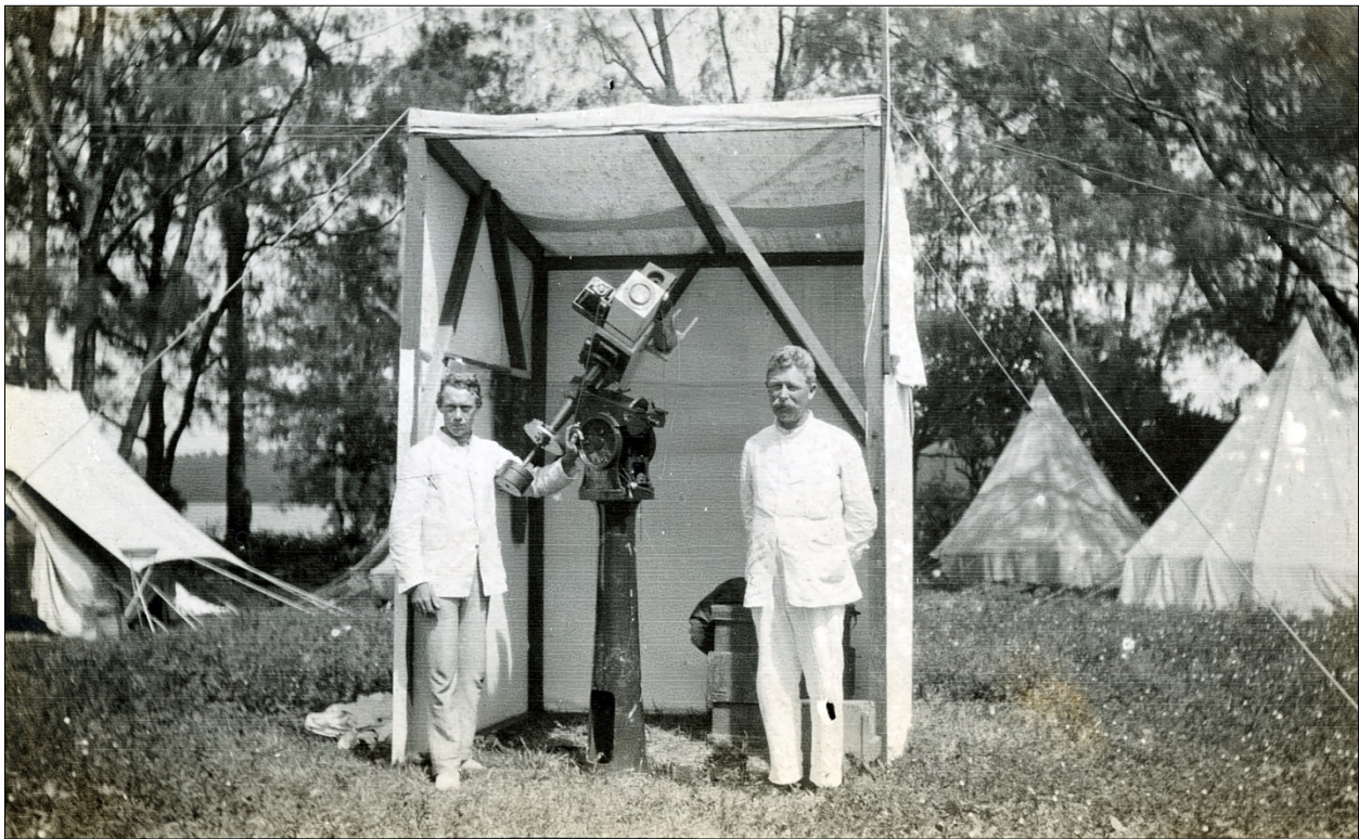
Figure 13: The Sydney University coronagraph and camera on a Grubb equatorial mount looked after by Rupert Holloway (left) and Richard Bulkeley (photograph: Thomas Baker, courtesy: State Library of South Australia, Dodwell Album, PRG 22/24 Volume 3).
