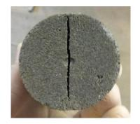
Figure 2. Sample tested for tension.
