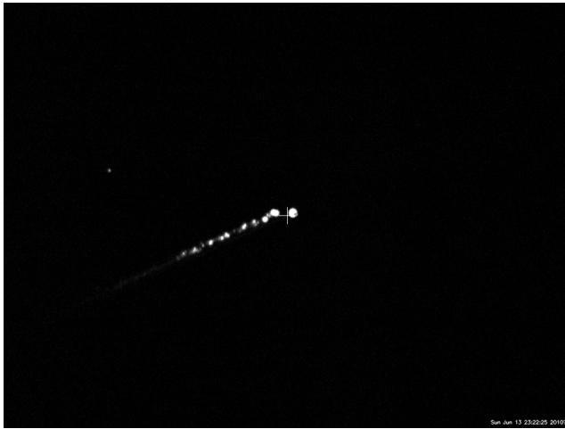
Fig. 15. On the left is one of the tracking images during the Hayabusa's reentry. Note that the target of interest is the re-entry capsule which is leading a trail of burning spacecraft. Image on the right shows the preliminary analysis of one of the spectral emission lines of the Hayabusa's re-entry capsule.
