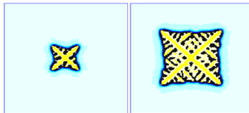
Figure 3. Effect of cooling rate on equiaxed dendrite growth for a given nucleus, t=0.63s , (a) 0.02 \text{ K/s} (b) 0.2 \text{ K/s}
