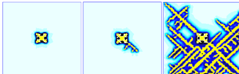
Figure 4. Growth of dendrite tip into undercooled melt through solute layer with a cooling rate 2 \text{ K/s} for a given nucleus, t=0.34, 0.36, 0.364s
