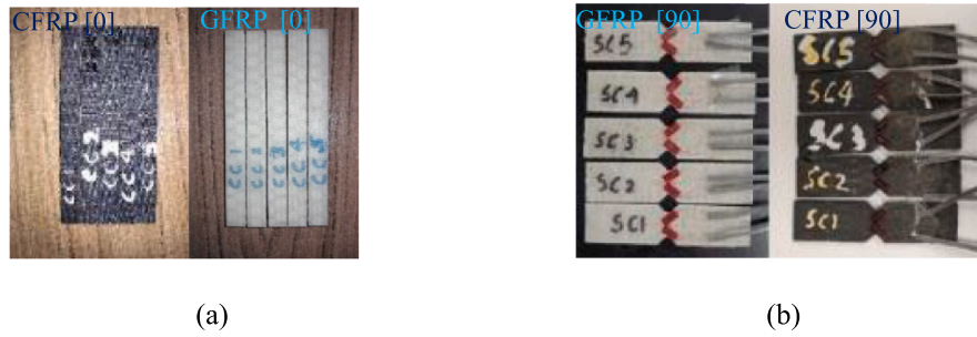
Fig. 3. (a) Compression test specimens; (b) Shear test specimens.
