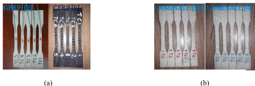
Fig. 2. (a) Tensile specimens of layer 1 & 2; (b) Tensile specimens of laminate.
