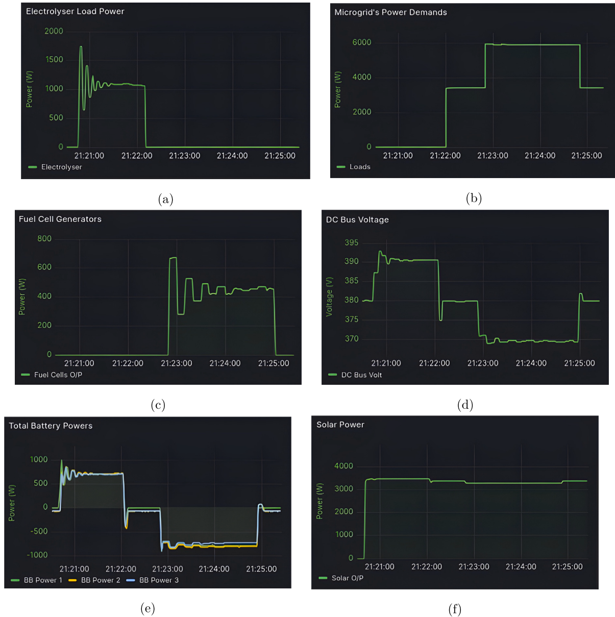
Fig. 10. Autonomous operation: (a) electrolyser, (b) loads, (c) fuel cells, (d) DC link, (e) battery banks, and (f) solar generation.
