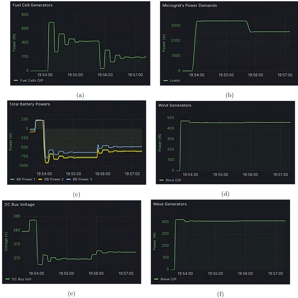
Fig. 8. Fuel cell's operation based on DC link voltage: (a) fuel cells, (b) loads, (c) battery banks, (d) wind generator, (e) DC link and (f) wave generator.
