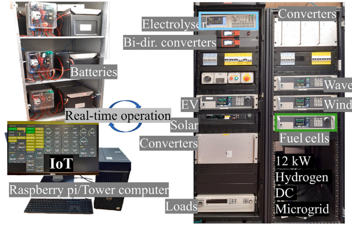
Fig. 5. The industry standard experimental set-up at Griffith University.
