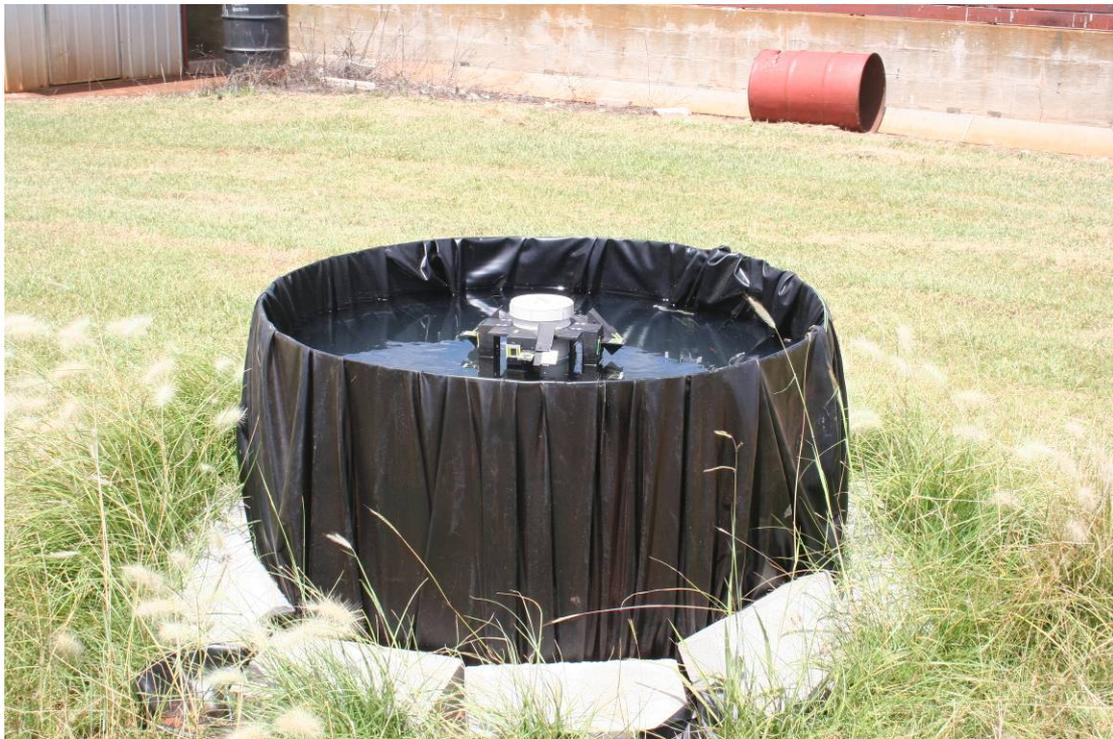
Figure 8.6: The simulated sea water environment located on the University of Southern Queensland campus grounds.
