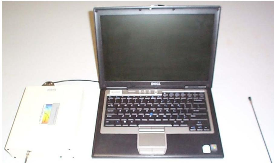
Figure 4.7: The EPP2000 spectrometer with a laptop computer used for data acquisition and the diffuser connected via a fibre optic link.
