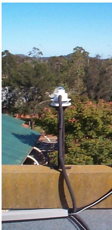
Figure 4.10: The Solar Light UV broadband meter.
