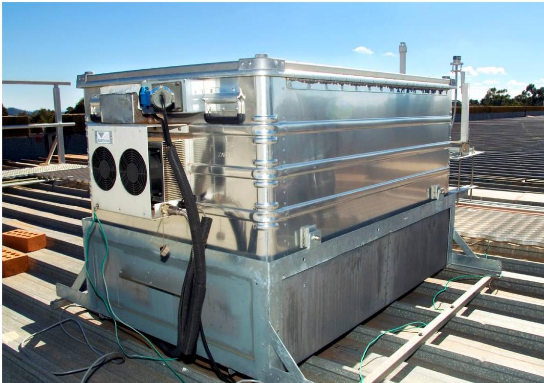
Figure 4.9: The Bentham spectroradiometer on the roof inside the Envirobox. The diffuser can be seen on the right hand side of the unit.
