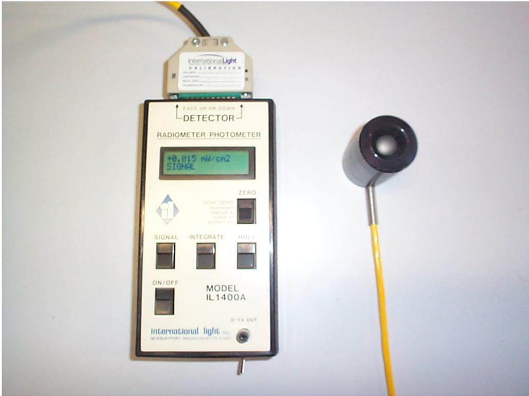
Figure 4.1: The International Light IL1400 broadband UVB meter with the waterproof detector.
