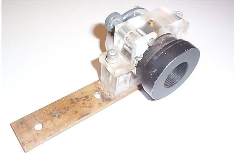
Figure 5.4: Dosimeter holder apparatus employed for the measurement of each PPO dosimeter.
