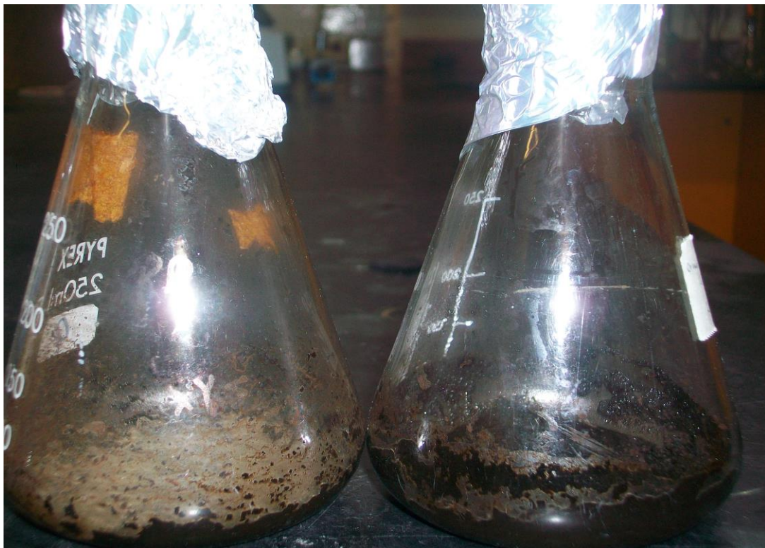
Figure 5.5: Solid state fermentation of coffee residues by Aspergillus awamori
