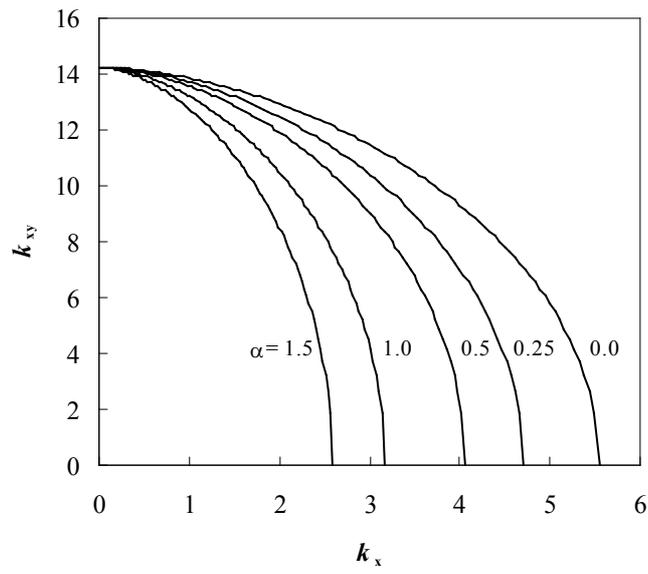
**Fig. 6.** Buckling interaction curves of plates (C-S-S-S+SC)
