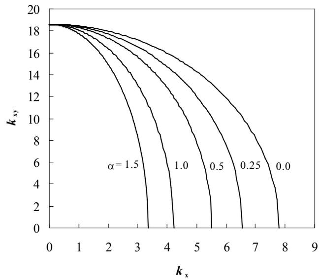
**Fig. 7.** Buckling interaction curves of plates (C-C-S-S+SC)
