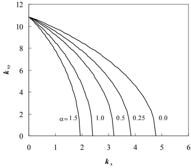
**Fig. 4.** Buckling interaction curves of plates (S-S-S-S+SC)
