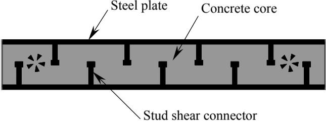
**Fig. 1.** Cross-section of double skin composite panel
