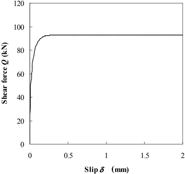
**Fig. 3.** Shear-slip curve for stud shear connectors
