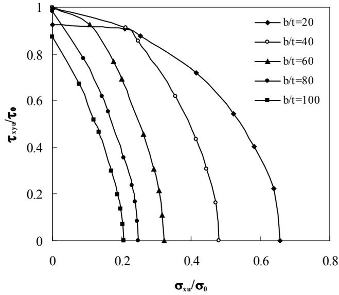
**Fig. 8.** Strength interaction curves of plates with various  $b/t$  ratios
