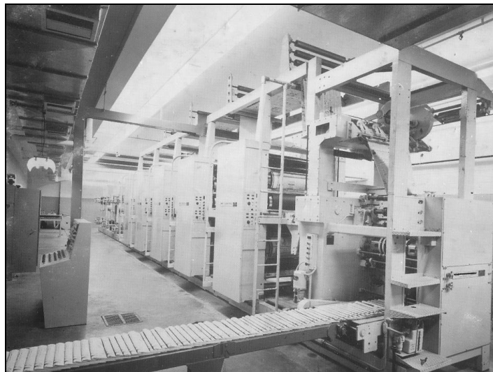
Figure 1.2 The Harris N845 offset newspaper printing as first installed at The Chronicle newspaper, Ruthven Street, and in use until 2008. Photograph – supplied by The Chronicle.
