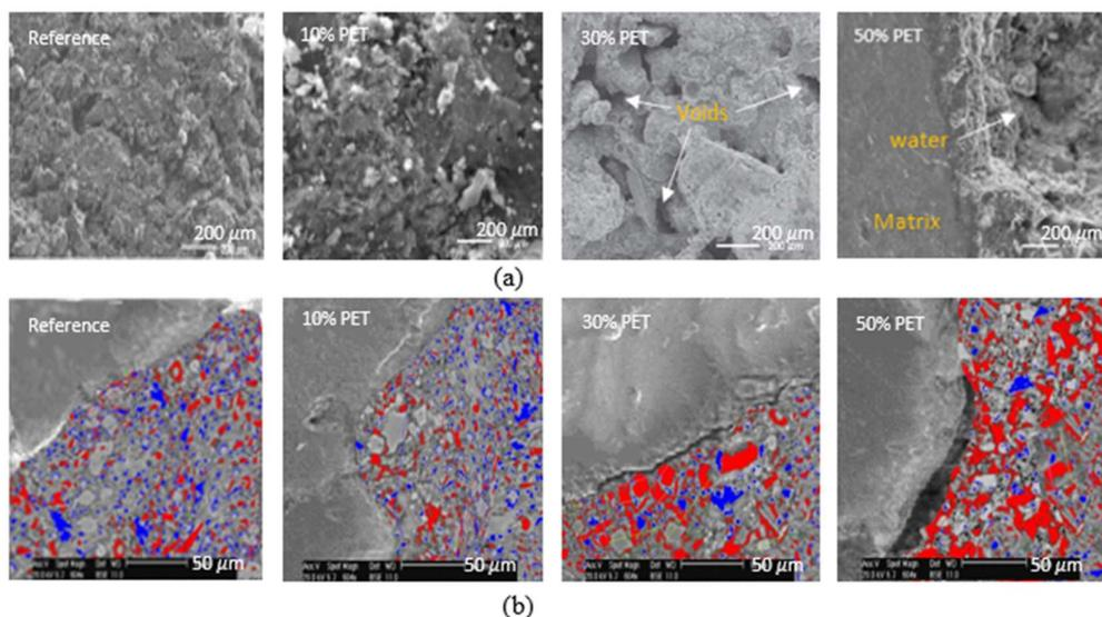
Fig 6 (a) Morphology and (b) porosity analysis of the specimens
