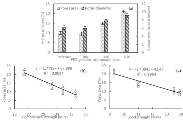
Fig. 7. (a) Pores area and diameter of the specimens, (b) correlation of pores area with compressive strength, and (c) bond strength.
