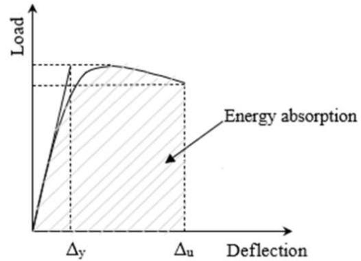
Fig. 9. Ductility and energy absorption measurements.
