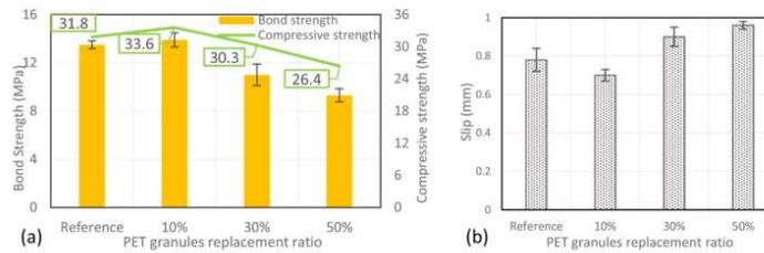
Fig. 4. Test results for (a) ultimate bond strength (b) ultimate slip.
