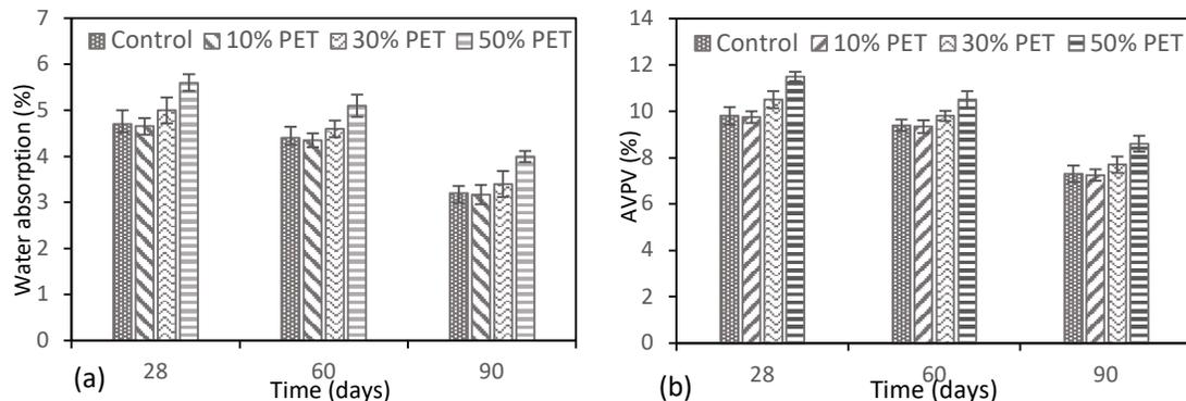
Figure 13 (a) Water absorption, (b) AVPV
