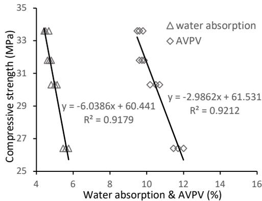
Figure 14 Relationship of compressive strength with AVPV and water absorption
