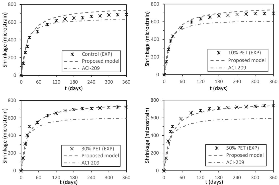
Figure 19 Comparison of experimental results with proposed model predictions
