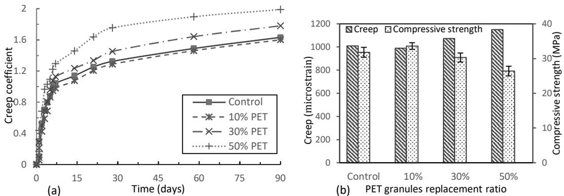
Figure 11 (a) creep coefficient, (b) creep strain and compressive strength of concrete mixes
