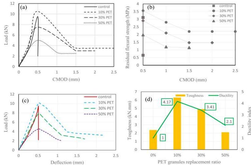
Fig. 9. Load-CMOD curves, (b) Residual flexural tensile strength results, (c) Load-deflection curves, (d) Toughness and ductility values.
