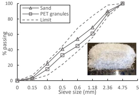
Figure 1 Grading curves for sand and PET granules
