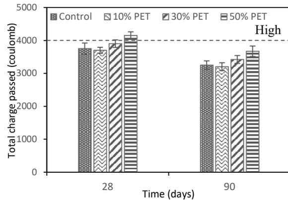
Figure 15 RCPT test results
