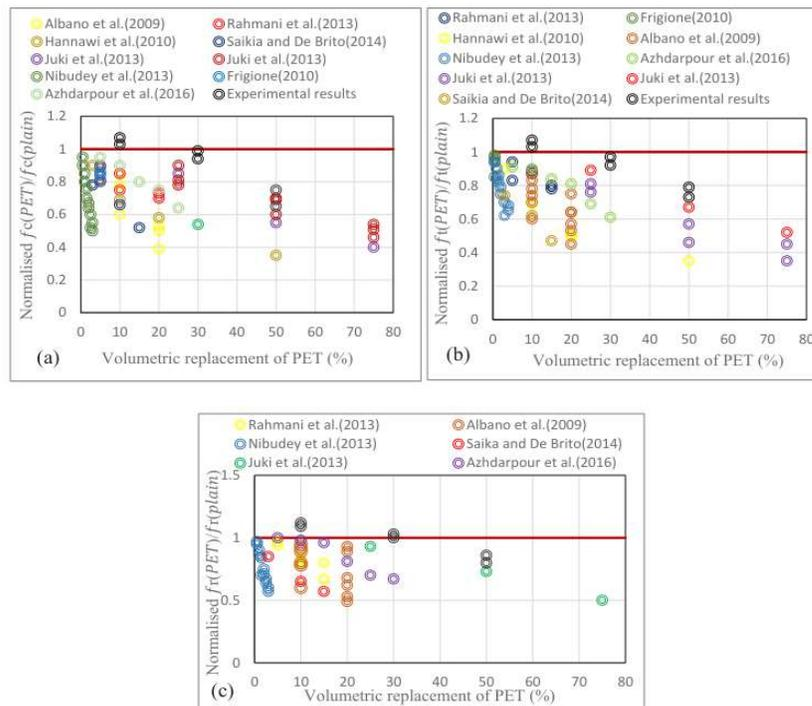
**Fig. 12.** Variation of the normalised properties with PET volume (a) compressive strength ( $f_c$ ), (b) tensile strength ( $f_t$ ), (c) flexural strength ( $f_r$ ).
