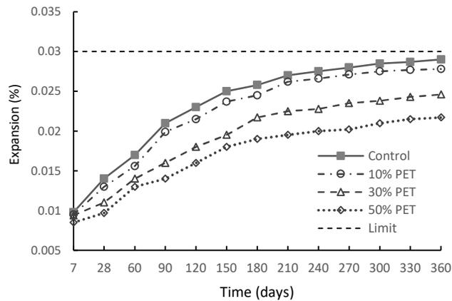
Figure 7 ASR expansion of concrete prisms.
