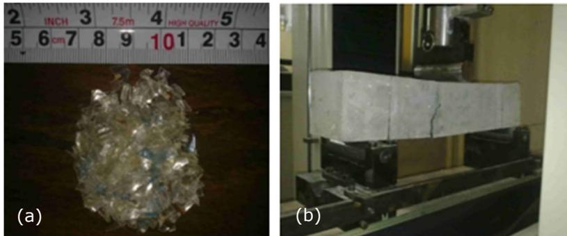
Figure 2.11 (a) PET particles, (b) flexural test (Rahmani et al., 2013)
