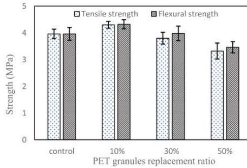
Fig. 7. Tensile and flexural test results.
