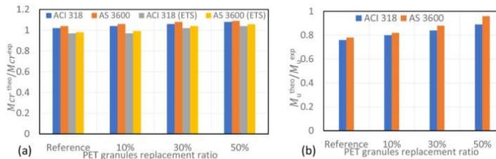
Fig. 11. Theoretical to experimental (a) cracking moment ratio (b) ultimate moment ratio.
