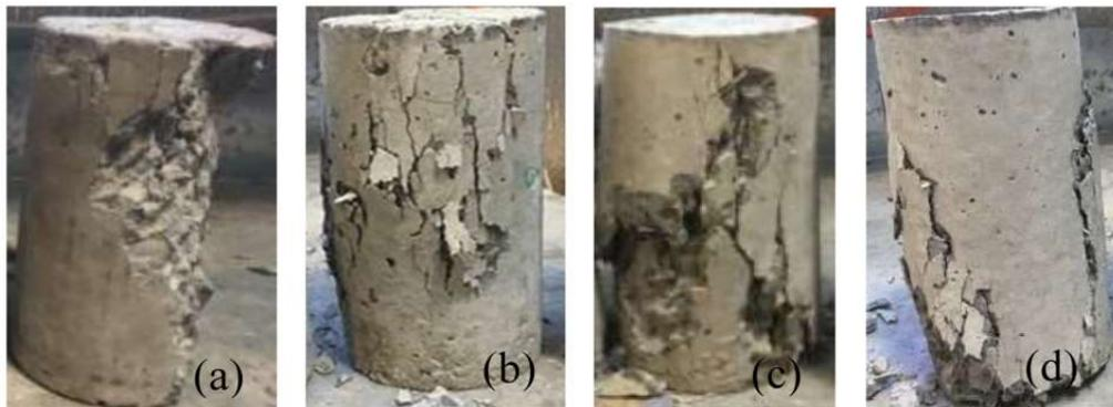
Fig. 5. Failure pattern of compressive strength test specimens: (a) control sample (b) 10% PET (c) 30% PET (d) 50% PET.
