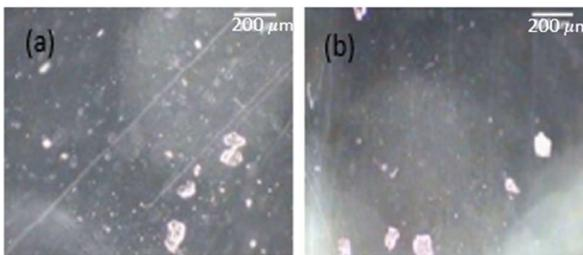
Figure 8 Surface morphology of PET granules in alkaline solution (a) 30 days, (b) 360 days
