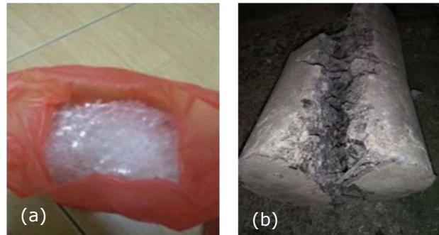
Figure 2.6 (a) PET fibres, (b) bridging effect of PET fibres (Shahidan, 2018)
