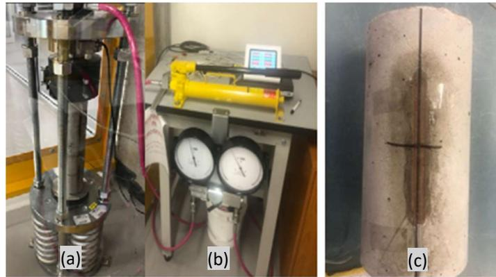
Figure 3 Creep test setup, (a) hydraulic spring-loaded machine, (b) Automated data collecting system, (c) specimen with strain gauge.
