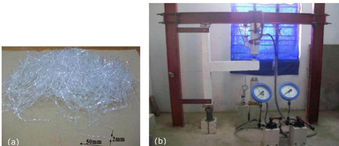
Figure 2.7 (a) straight slit PET fibres, (b) test set up (Marthong & Marthong, 2016)
