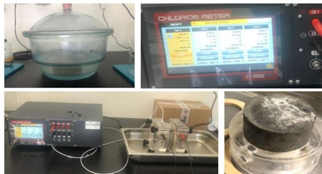
Figure 6 RCPT setup
