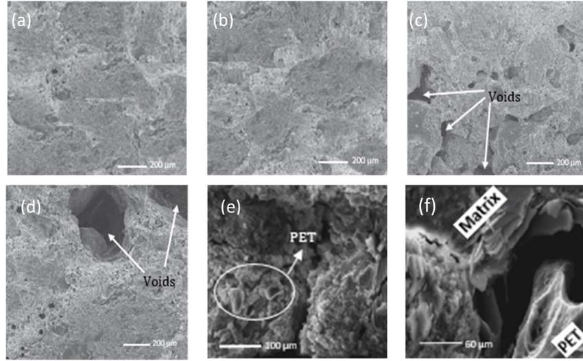
Figure 16 SEM images of (a) control, (b) 10% PET, (c) 30% PET, (d, e, f) 50% PET
