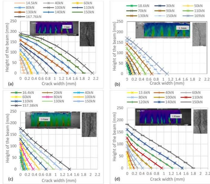
Fig. 10. Main crack propagation (a) reference beam, (b) 10% PET beam, (c) 30% PET beam, (d) 50% PET beam.
