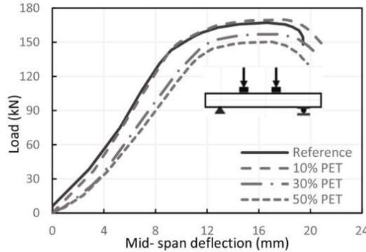
Fig. 8. Experimental load-deflection curves.
