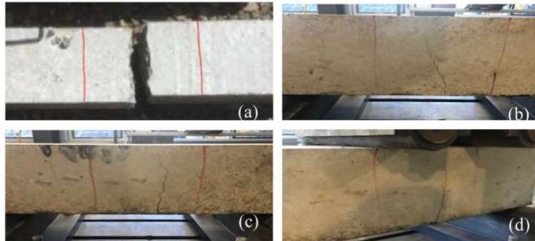
Fig. 8. Failure pattern of flexural strength test specimens: (a) control sample (b) 10% PET (c) 30% PET (d) 50% PET.
