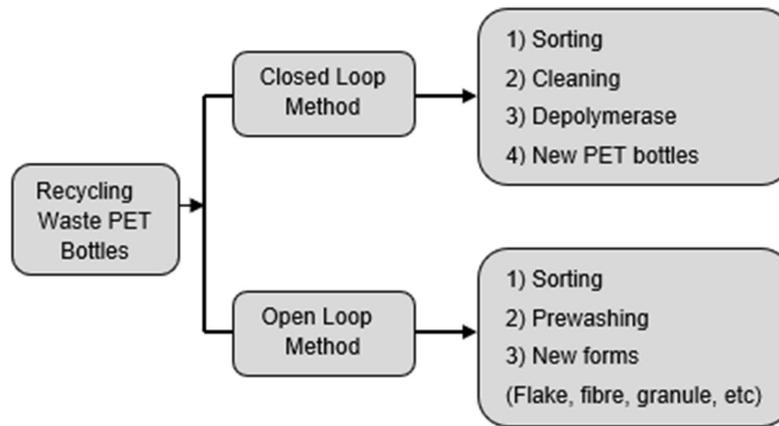
Figure 2.3 Recycling procedures of waste PET bottles (Andrady, 2015)
