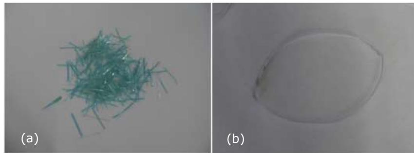
Figure 2.8 (a) short lamellar fibres, (b) O-shaped fibres (Foti, 2011)
