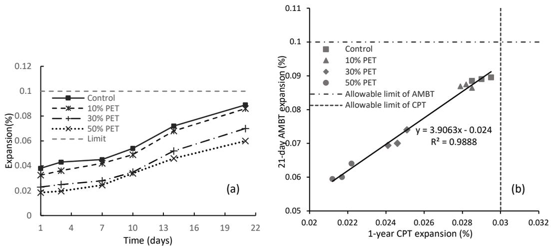
Figure 10 (a) ASR expansion of mortar bars, (b) Relationship between CPT and AMBT
