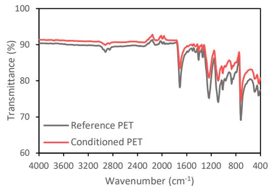
Figure 9 FTIR spectra of PET granule
