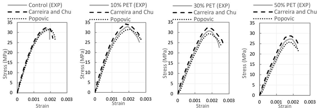
**Figure 2. Comparison of experimental stress-strain behavior with Carreira and Chu (1985) and Popovics (1973) models.**
