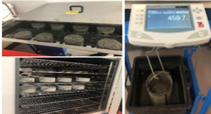
Figure 5 water absorption test setup
