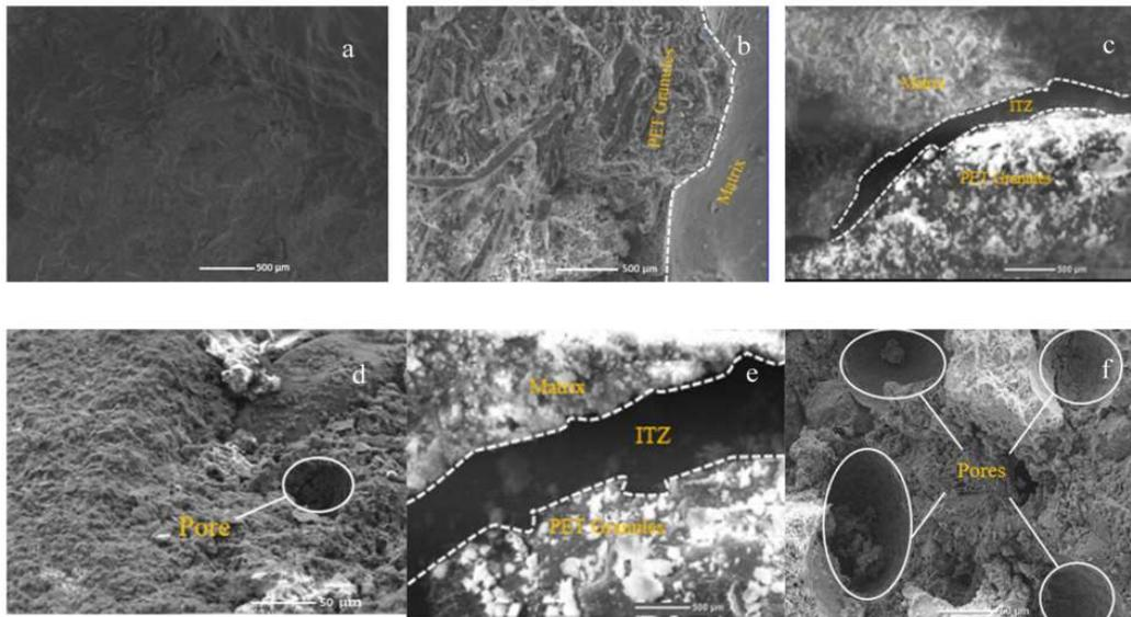
Fig. 11. SEM images (a) Control sample, (b) 10% PET, (c, d) 30% PET, (e, f) 50% PET.
