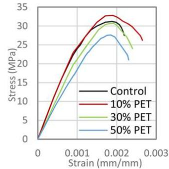
Fig. 2. Stress-strain behaviour.
