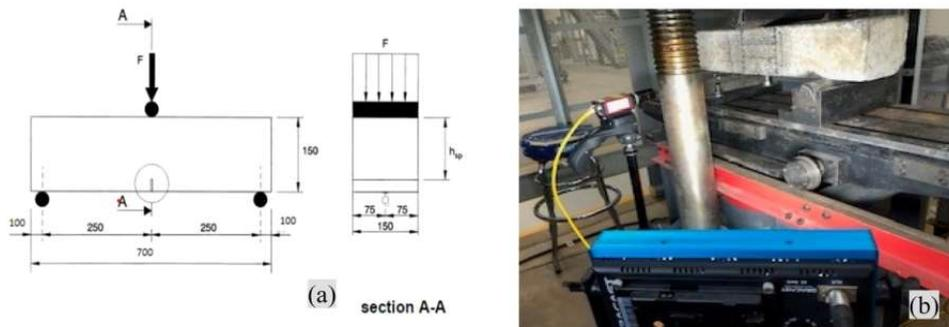
Fig. 3. (a) CMOD test schematic (BS-EN 14651–2005 [28]), (b) example of DIC set up.
