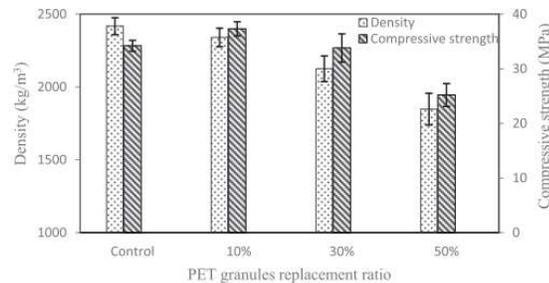
Fig. 4. Density and compressive strength results.
