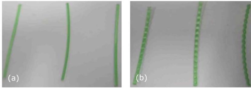
Figure 2.5 (a) straight fibres, (b) crimped fibres (Asha & Resmi, 2015)
