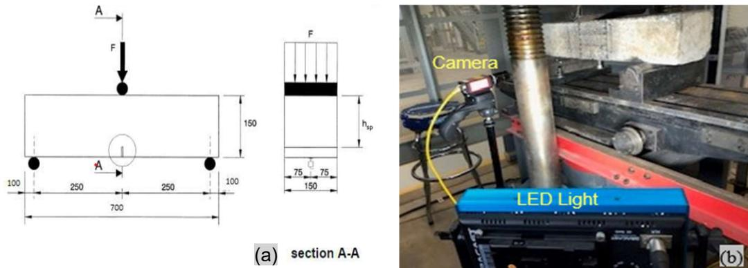
Fig 3. (a) CMOD test schematic (BS-EN 14651-2005 [28]), (b) example of DIC set
