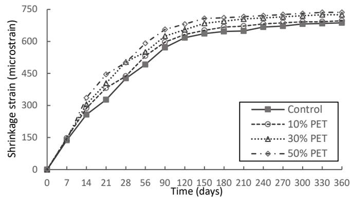
Figure 12 Shrinkage strain of the concrete mixtures
