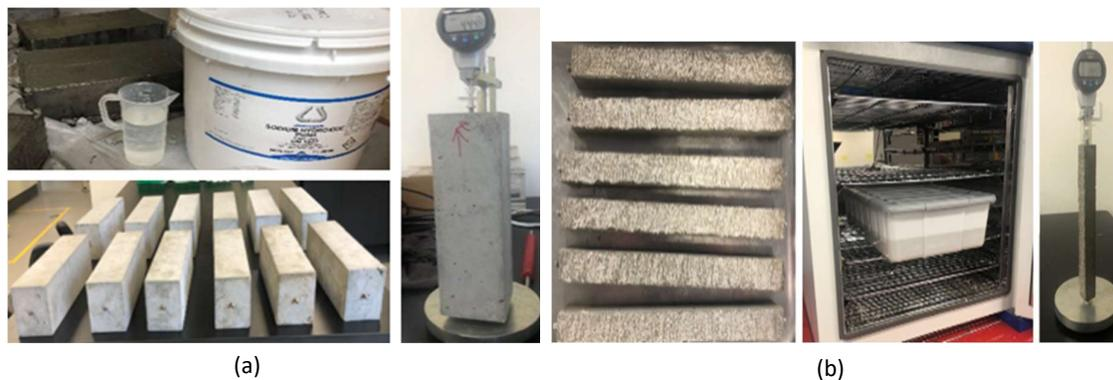
Figure 2 ASR test setup (a) CPT, (b) AMBT
