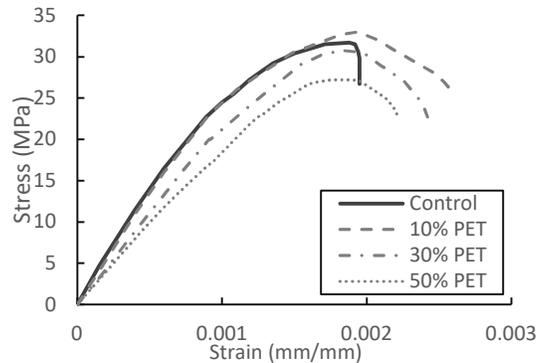
Figure1. Stress-strain behaviour of the concrete mixtures.
