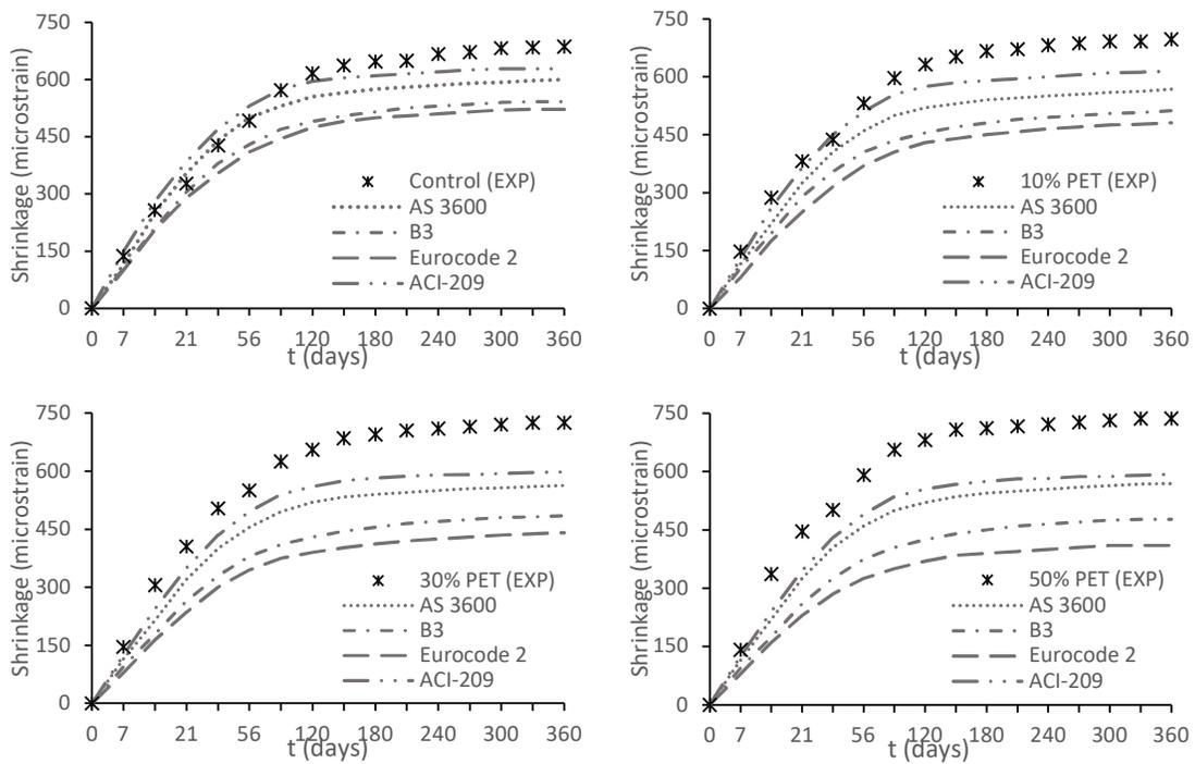
Figure 17 Comparison of current prediction models with experimental results
