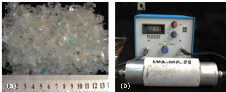
Figure 2.13 (a) sheet-shaped PET, (b) ultrasound test (Azhdarpour et al., 2016)
