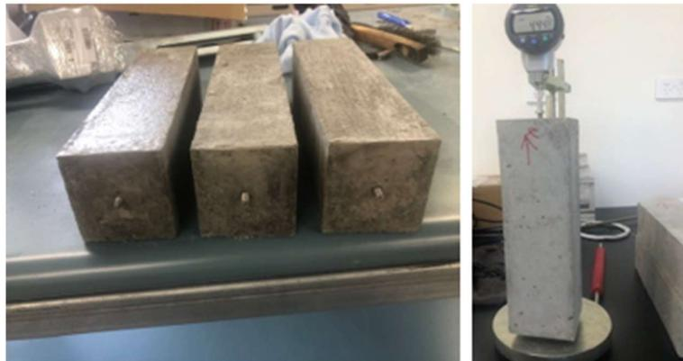
Figure 4 Shrinkage test setup
