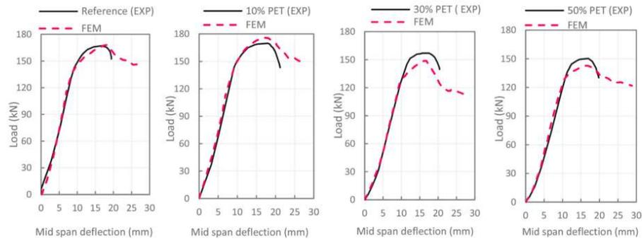
Fig. 13. Comparison between numerical and experimental load deflections.
