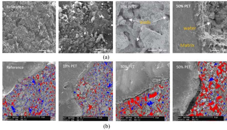
Fig. 6. (a) Morphology, and (b) porosity analysis of the specimens.
