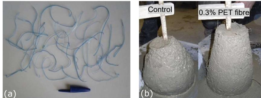
Figure 2.4 (a) PET fibres from waste bottle, (b) slump test (Wiliński et al., 2016).
