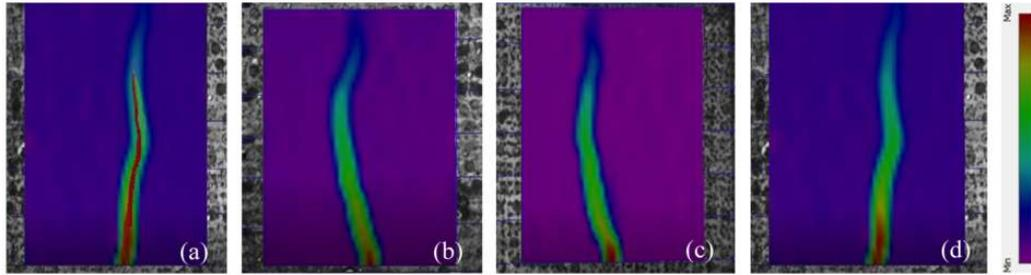
Fig. 10. Evolution of strain map for the crack path detection of the specimens: (a) control sample, (b) 10% PET, (c) 30% PET, (d) 50% PET.
