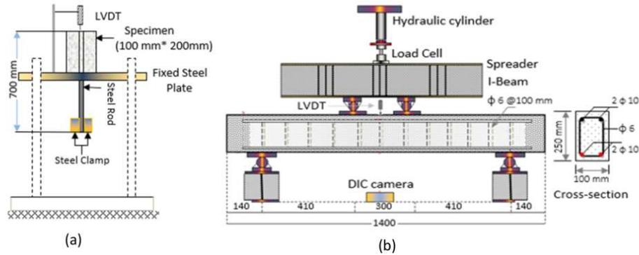
Fig. 1. Schematic diagram, (a) pull out test, (b) four point-bending test.
