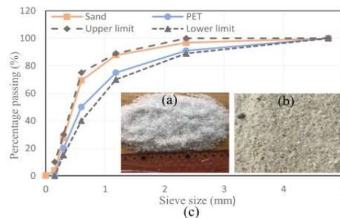
Fig. 1. (a) Recycled PET granules, (b) Sand, (c) Particle size distribution for sand, PET granules, AS 2758.1 [25].
