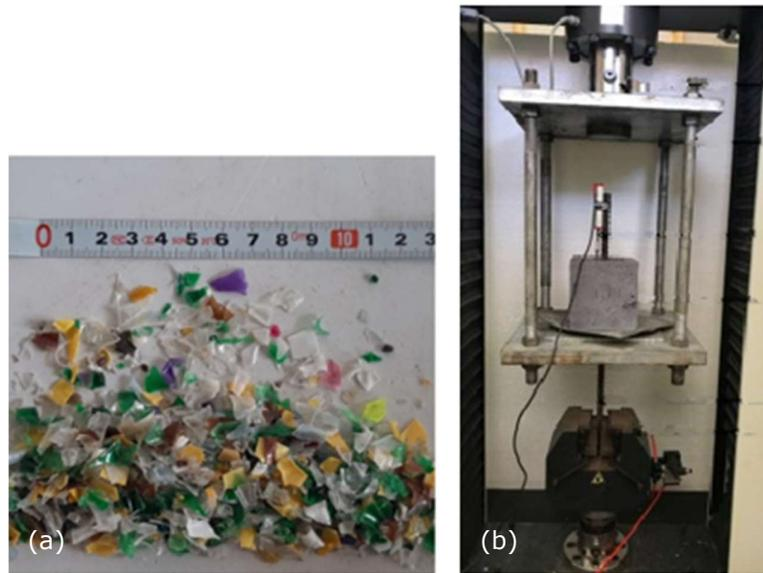
Figure 2.12 (a) shredded PET, (b) Pull-out test (Fakoor & Nematzadeh, 2021)
