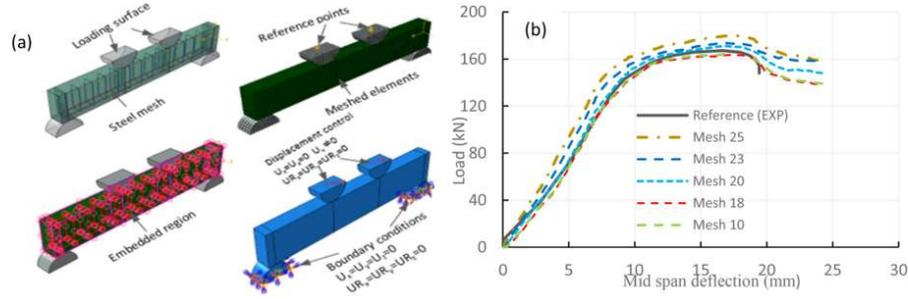
Fig. 12. (a) Geometry of FEM models, (b) mesh analysis.
