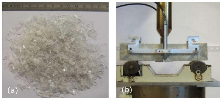
Figure 2.10 (a) PET aggregates, (b) flexural test (Hannawi et al., 2010)
