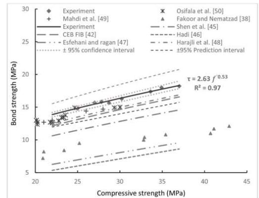
Fig. 5. Relationship between experimental results and predicted bond strength.
