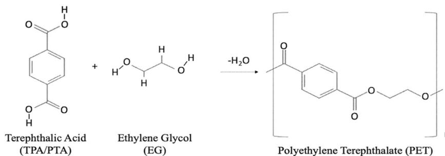
Figure 2.2 Formation of Polyethylene terephthalate (PET) (Benyathiar et al., 2022)
