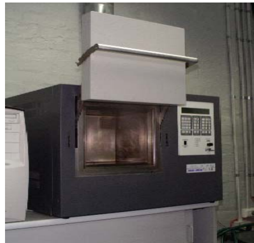
Figure 2: Cavity of VW 1500 Model with Frequency range of 6 -18 GHz and a Maximum Power of 125 W
