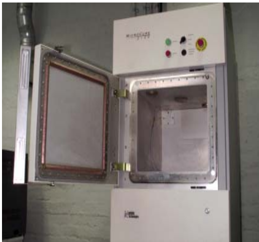
Figure 1: Cavity of Microcure 2100 Model 250 with Frequency Range of 2 - 7 GHz and a Maximum Power of 250 W
