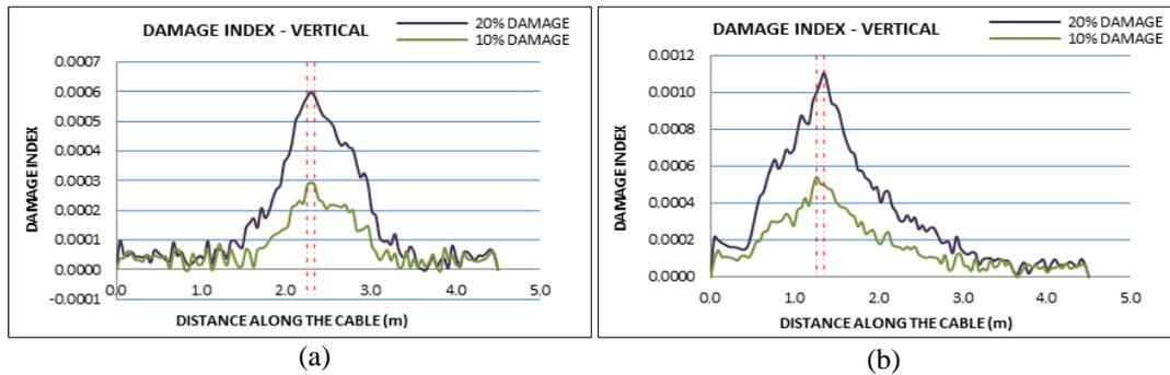
Fig. 21. Damage detection in TSC1 with 0.09m (2%) damage length with 10% and 20% stiffness reductions
