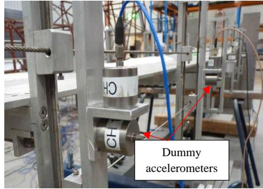
Fig. 5. Dummy accelerometers
