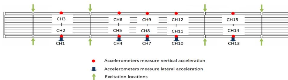
Fig. 4. Accelerometer layout and excitation locations in the plan view of bridge deck
